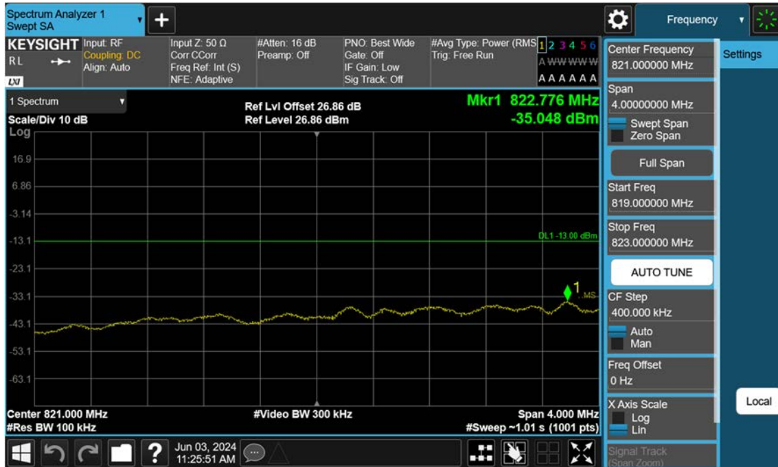
Sub6 n5_5 M_Extended Band Edge_Low_BPSK_FullIRB
