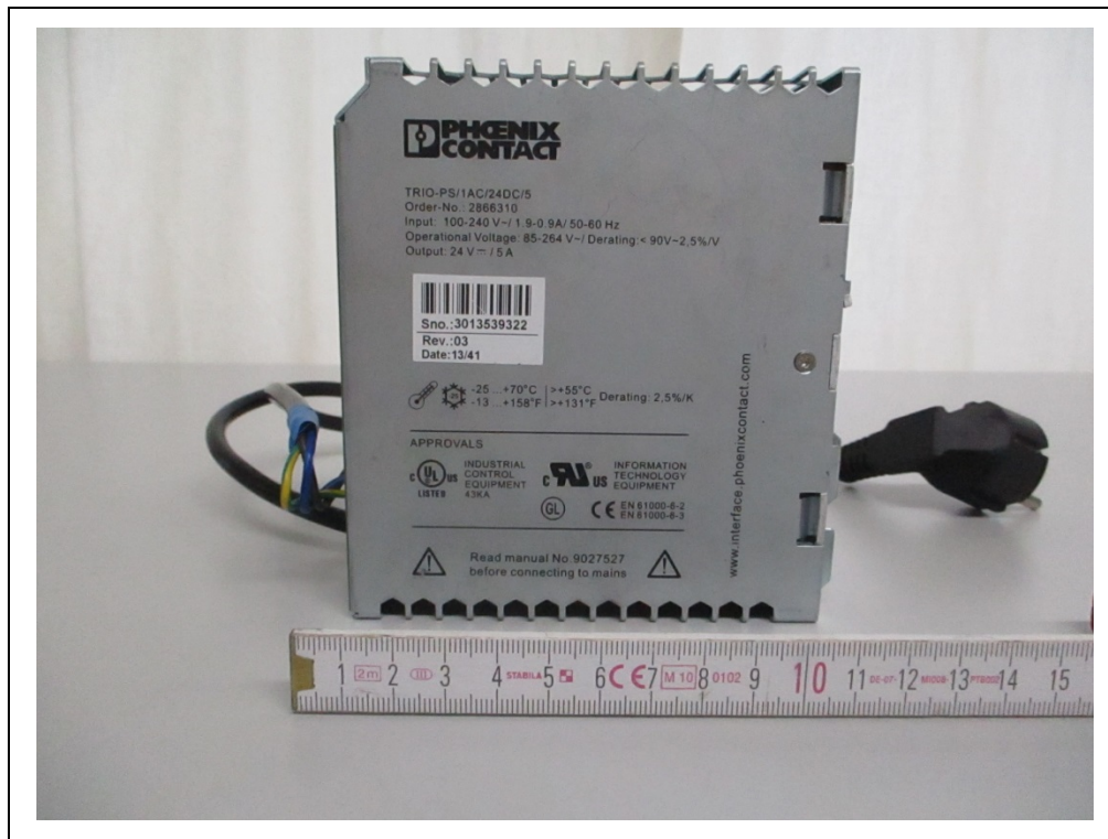
Photograph A3-7: Power supply TRIO-PS/1AC/24DC/5
