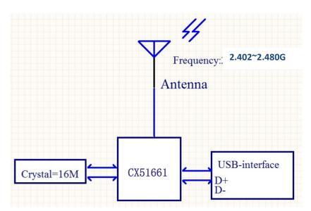
U1:The CX51661 solution is to use the mouse 2.4G COMPX new highly integrated IC , hardware integration USB controller,RF circuit, LDO, Voltage detector ...and other components, The CX51661 operates USB wireless mouse/keyboard device transceiver SOC.
