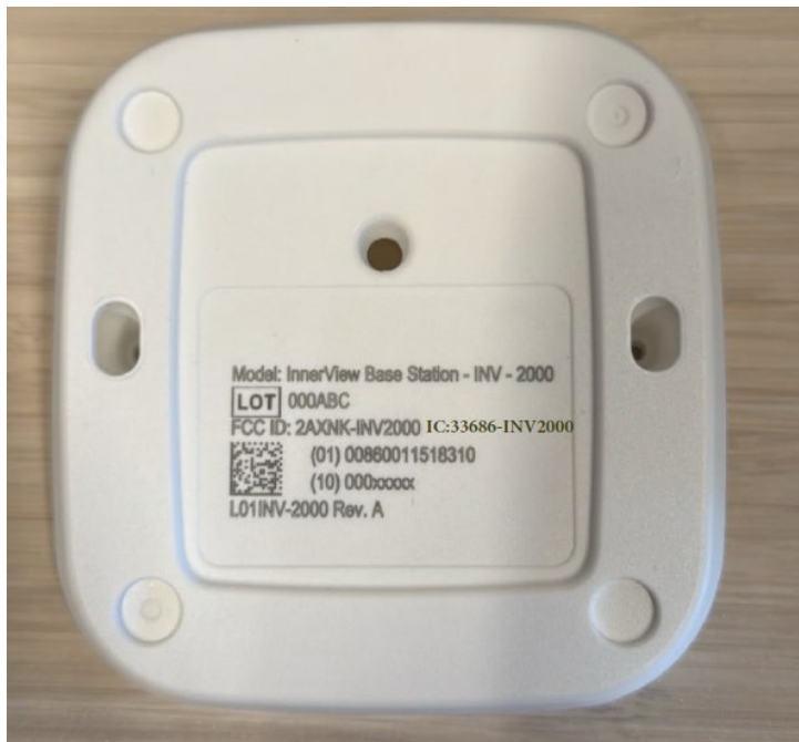
Image 1 – FCC /IC label on the bottom of the base station
