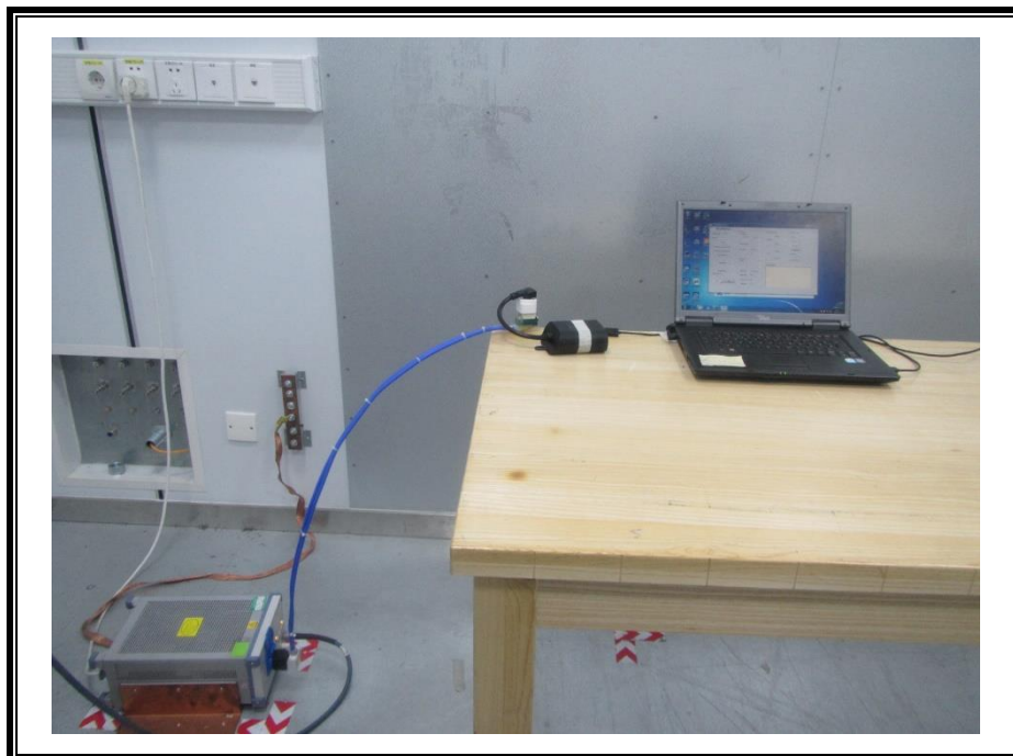
POWERLINE CONDUCTED EMISSIONS MEASUREMENT SETUP
