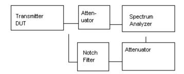
Method of Measuring Conducted Spurious Emissions
