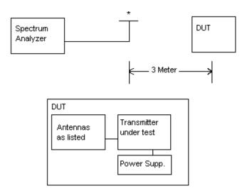
Equipment placed 80cm above ground on a rotatable platform.
