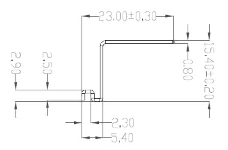
Figure 1 Physical dimension (mm)
