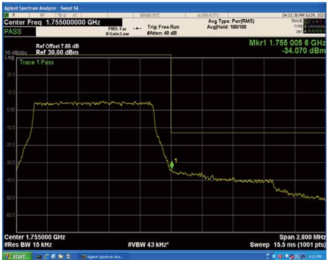
Band4 QAM16 BW=1.4MHz Channel=20393 RB Size=1 Position=#0
