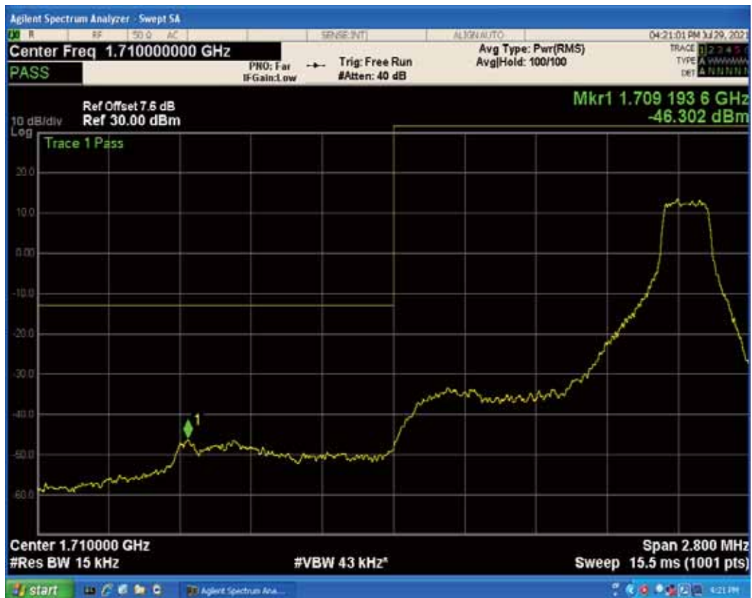
Band4 QPSK BW=1.4MHz Channel=19957 RB Size=1 Position=#0
