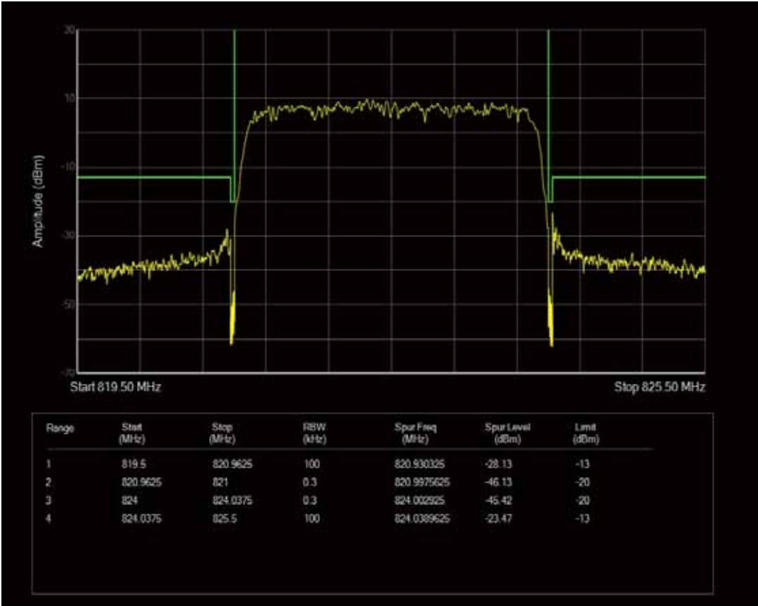
Band26a QAM16 BW=3MHz Channel=26775 RB Size=1 Position=#0
