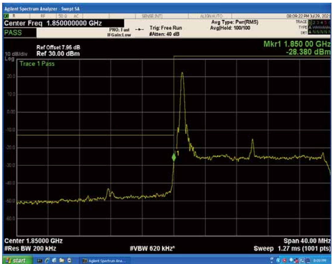
Band25 QPSK BW=20MHz Channel=26140 RB Size=100 Position=#0
