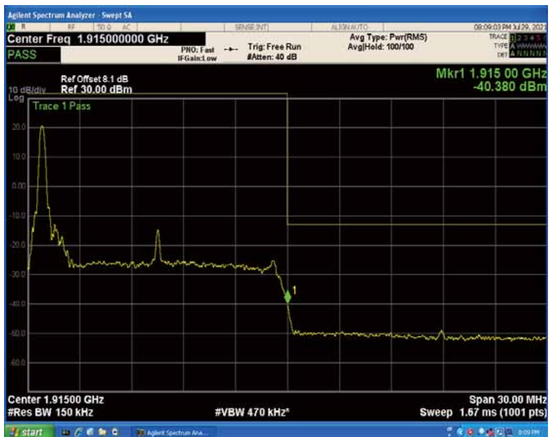
Band25 QAM16 BW=15MHz Channel=26615 RB Size=1 Position=#Max
