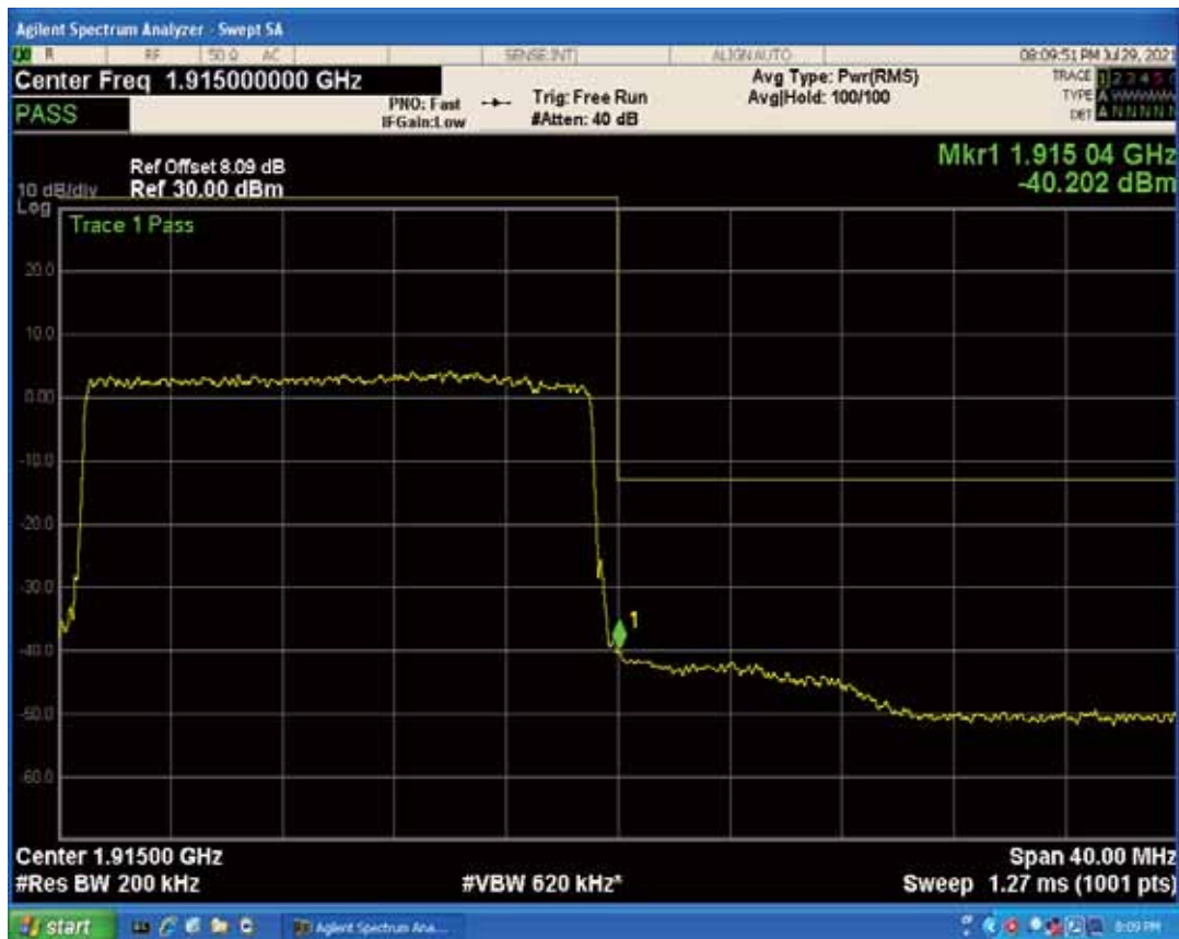
Band25 QAM16 BW=20MHz Channel=26590 RB Size=1 Position=#0
