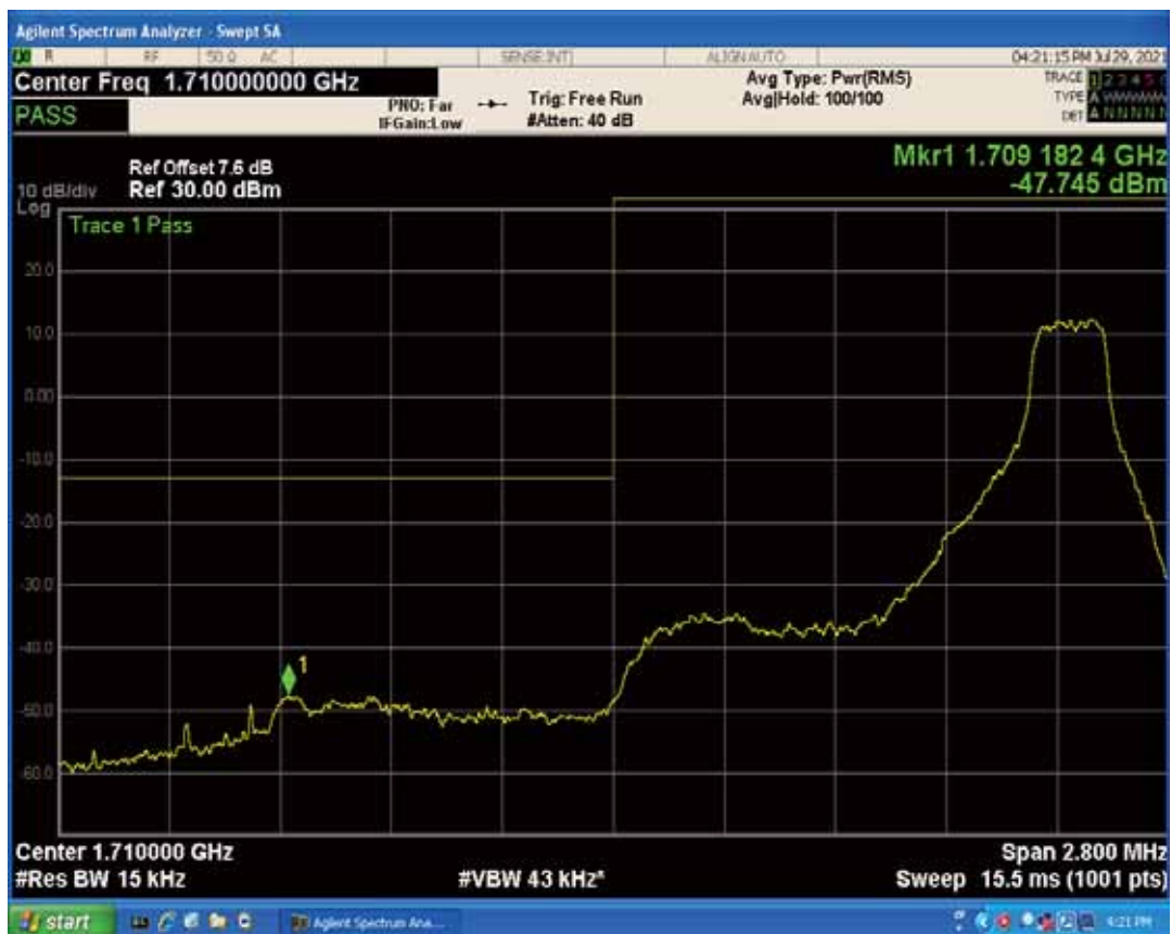
Band4 QAM16 BW=1.4MHz Channel=19957 RB Size=6 Position=#0
