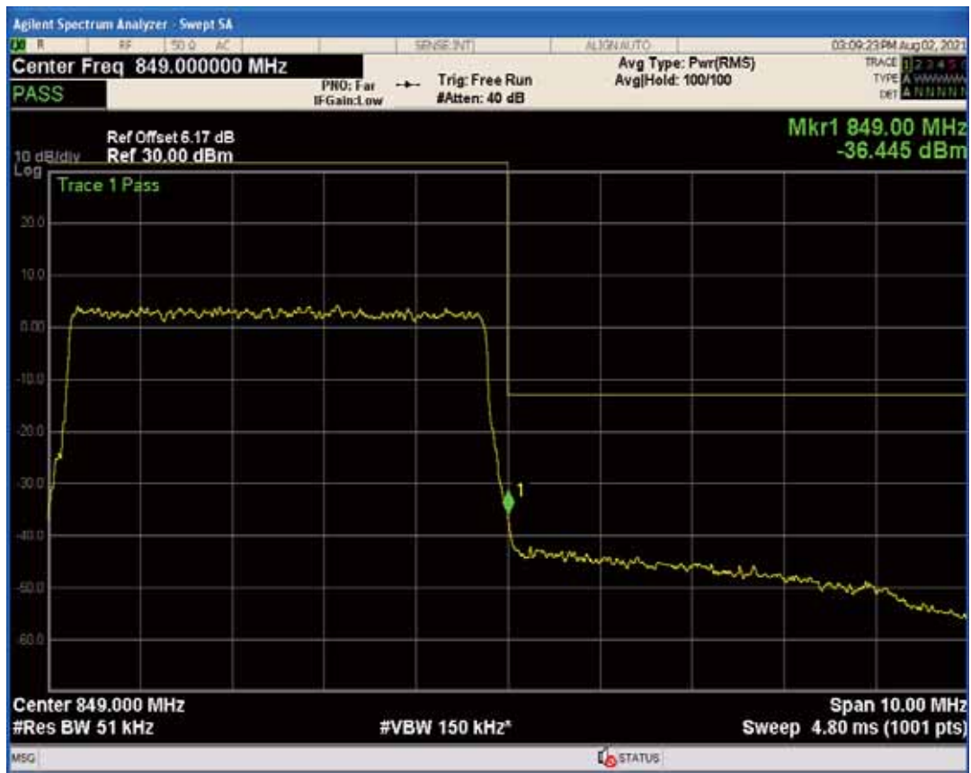
Band26b QAM16 BW=5MHz Channel=27015 RB Size=1 Position=#0
