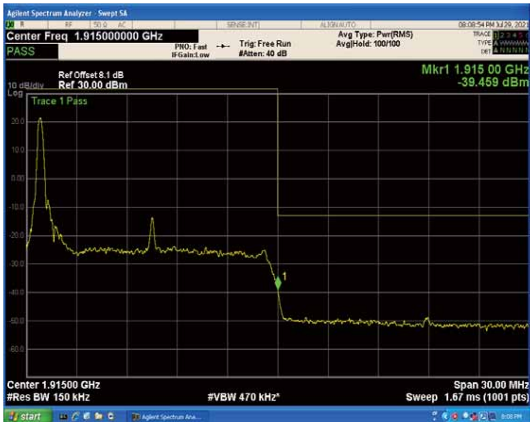
Band25 QPSK BW=15MHz Channel=26615 RB Size=1 Position=#Max
