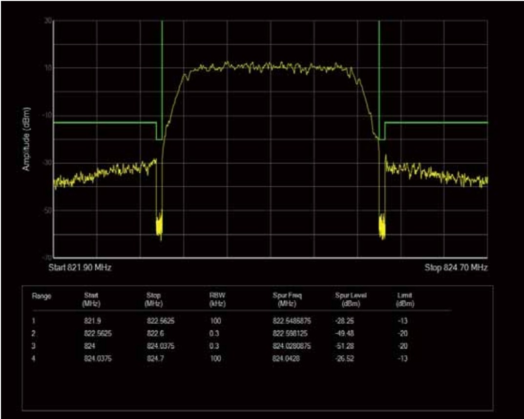
Band26a QAM16 BW=1.4MHz Channel=26783 RB Size=1 Position=#Max
