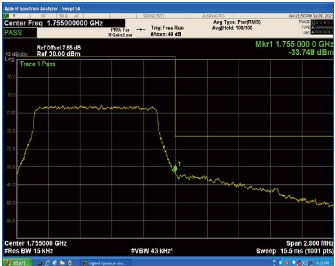
Band4 QPSK BW=3MHz Channel=19965 RB Size=1 Position=#Max
