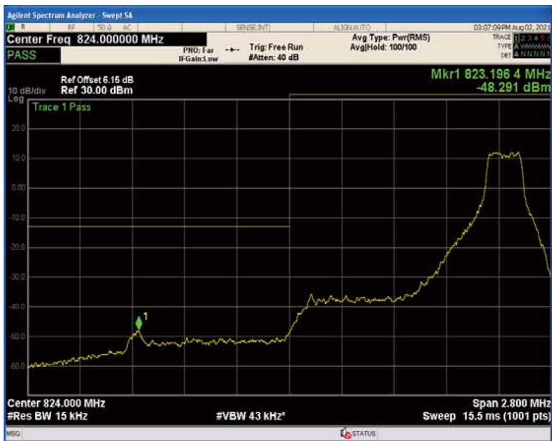
Band26b QPSK BW=1.4MHz Channel=27033 RB Size=1 Position=#0
