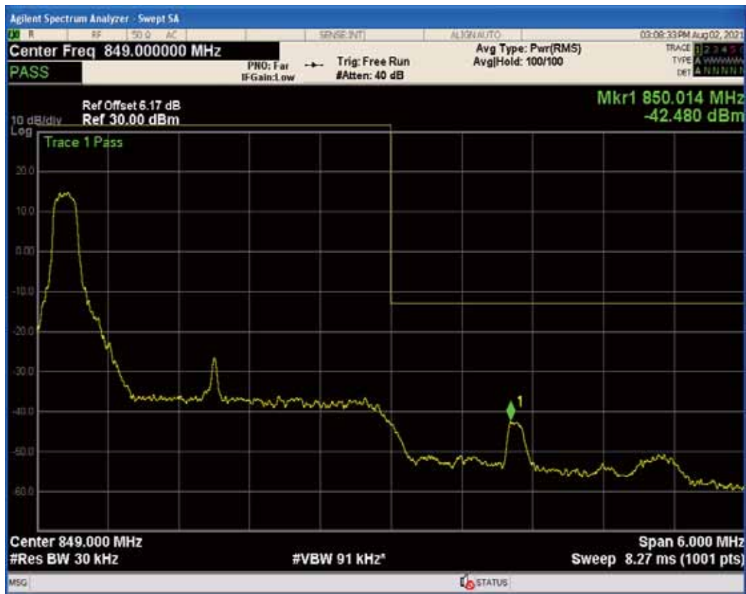
Band26b QPSK BW=5MHz Channel=26815 RB Size=1 Position=#0
