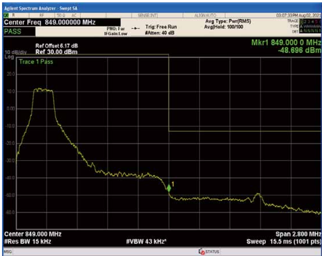
Band26b QAM16 BW=1.4MHz Channel=27033 RB Size=1 Position=#Max
