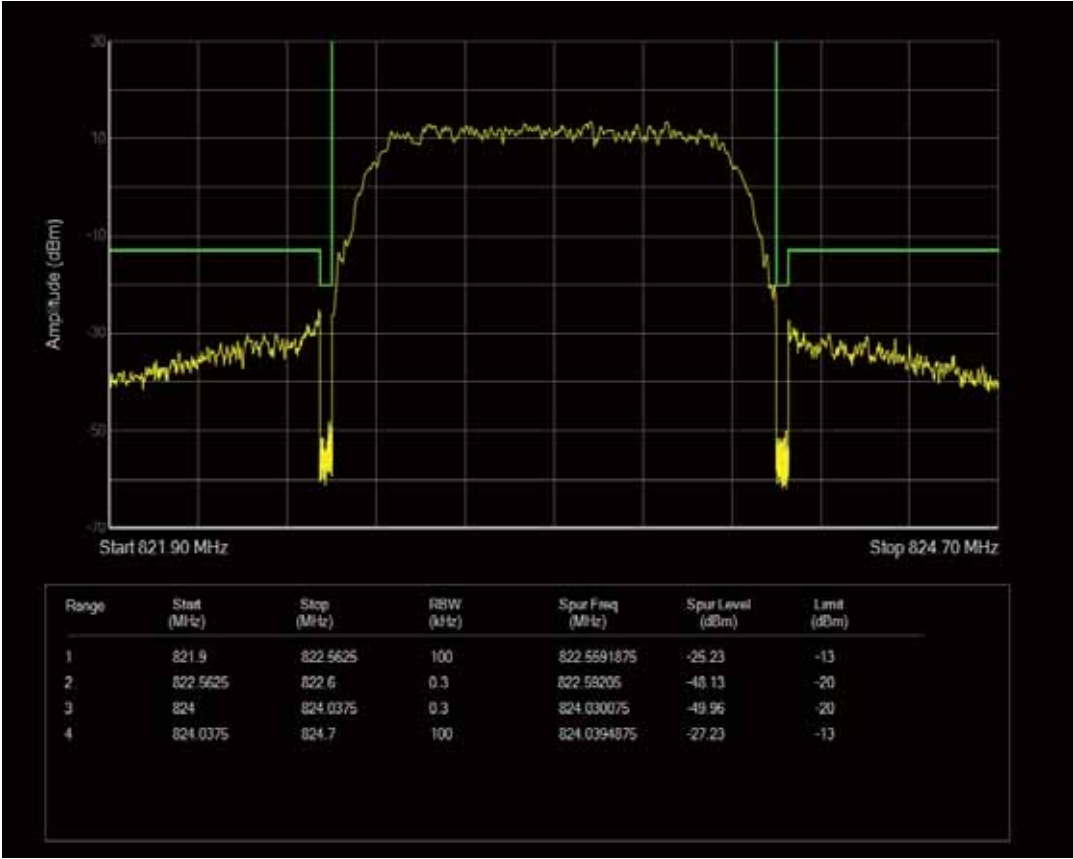
Band26a QPSK BW=1.4MHz Channel=26783 RB Size=1 Position=#Max
