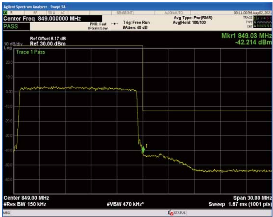
Band26b QAM16 BW=15MHz Channel=26965 RB Size=1 Position=#Max
