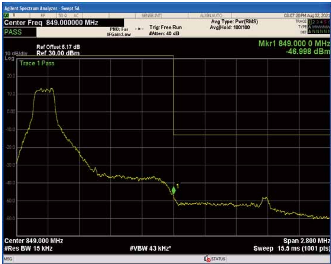
Band26b QPSK BW=1.4MHz Channel=27033 RB Size=1 Position=#Max
