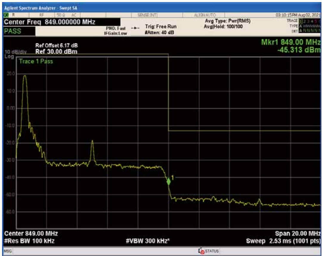
Band26b QAM16 BW=10MHz Channel=26990 RB Size=50 Position=#0
