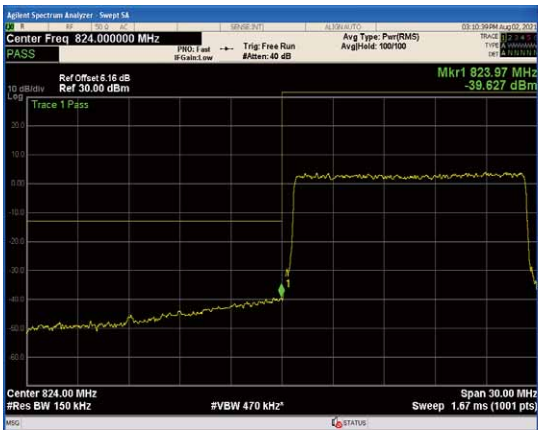
Band26b QAM16 BW=15MHz Channel=26865 RB Size=1 Position=#0
