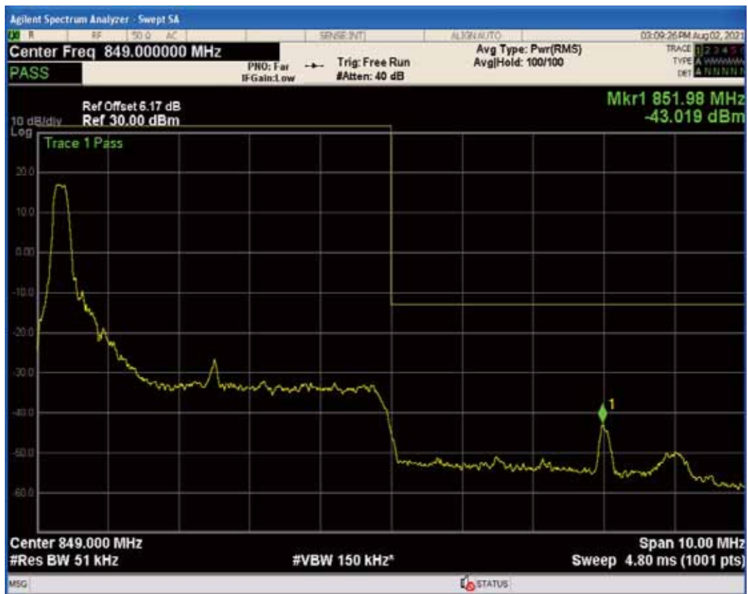
Band26b QAM16 BW=5MHz Channel=27015 RB Size=25 Position=#0
