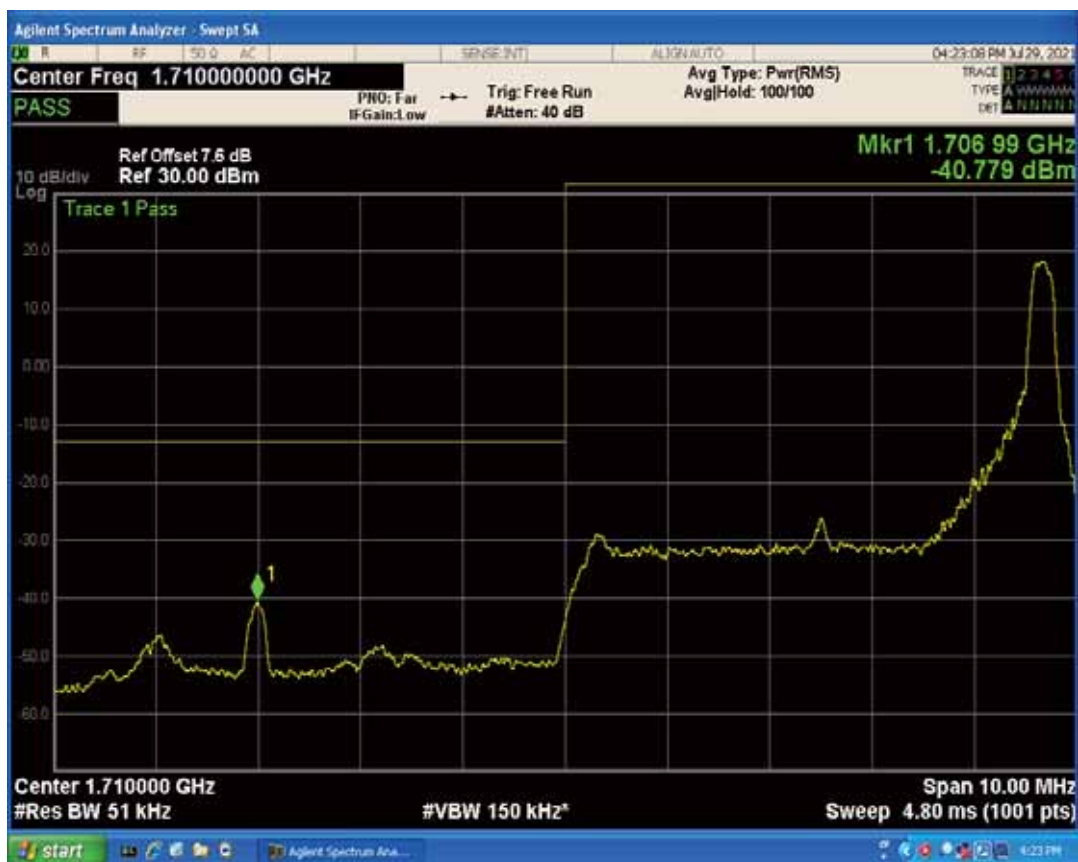
Band4 QAM16 BW=5MHz Channel=19975 RB Size=1 Position=#0
