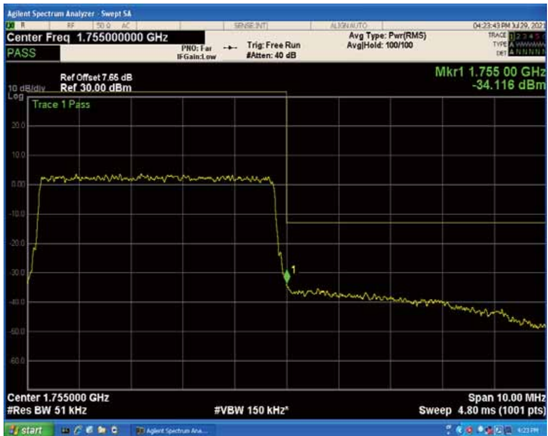
Band4 QPSK BW=10MHz Channel=20000 RB Size=1 Position=#Max
