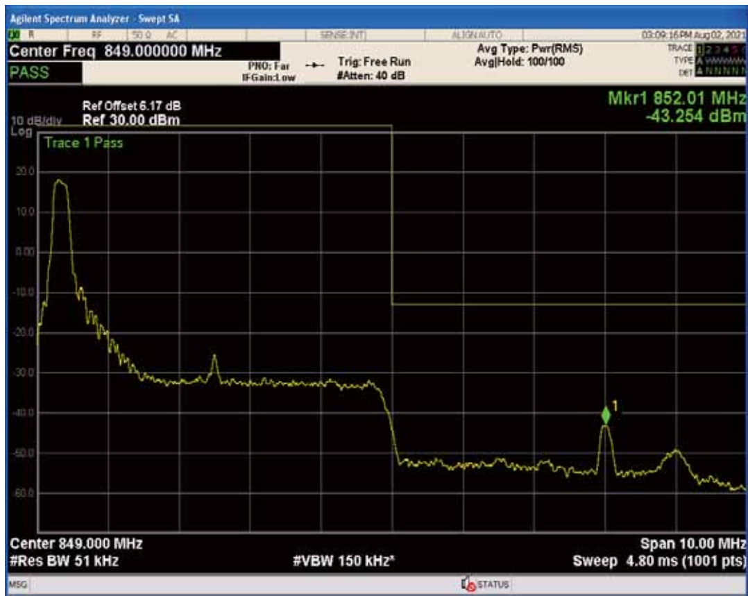
Band26b QPSK BW=5MHz Channel=27015 RB Size=1 Position=#Max
