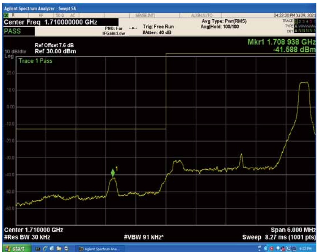
Band4 QAM16 BW=3MHz Channel=19965 RB Size=15 Position=#0
