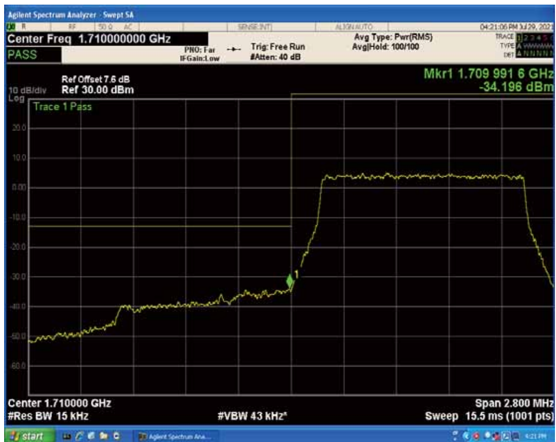
Band4 QAM16 BW=1.4MHz Channel=19957 RB Size=1 Position=#0
