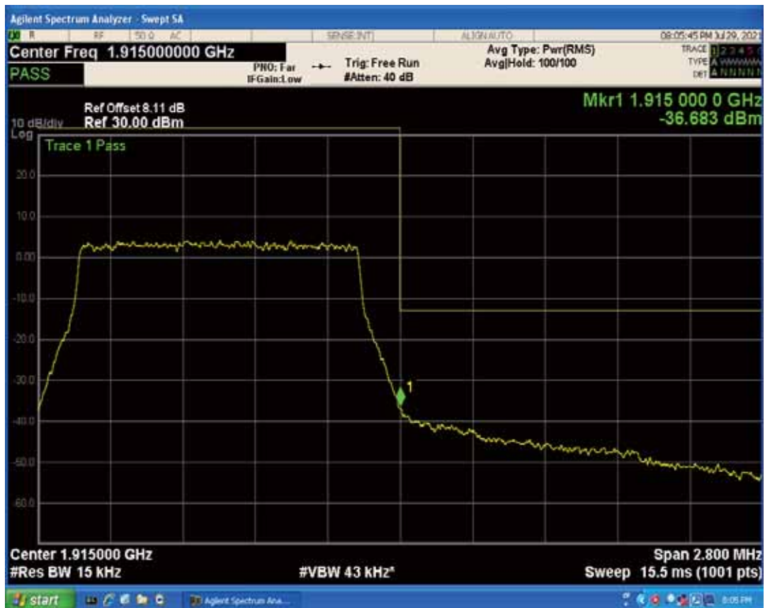
Band25 QPSK BW=3MHz Channel=26055 RB Size=1 Position=#Max
