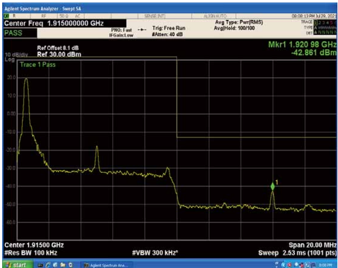
Band25 QAM16 BW=10MHz Channel=26640 RB Size=1 Position=#Max
