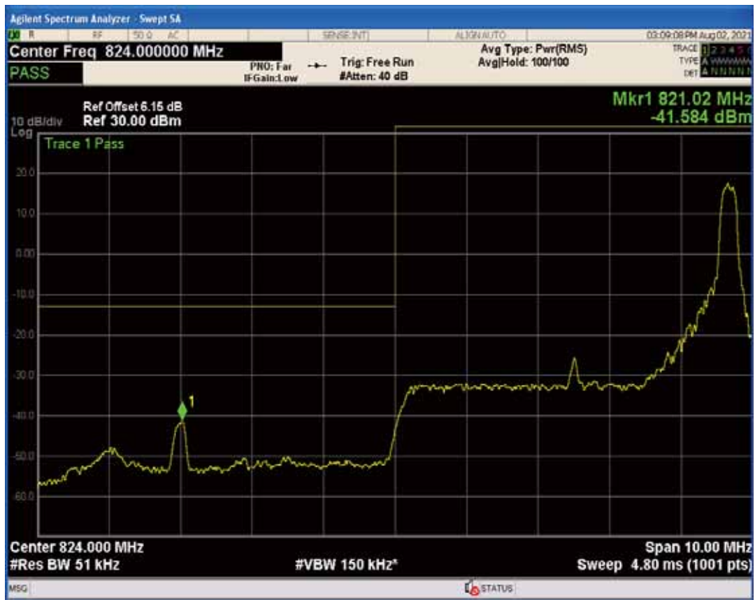
Band26b QAM16 BW=5MHz Channel=26815 RB Size=25 Position=#0
