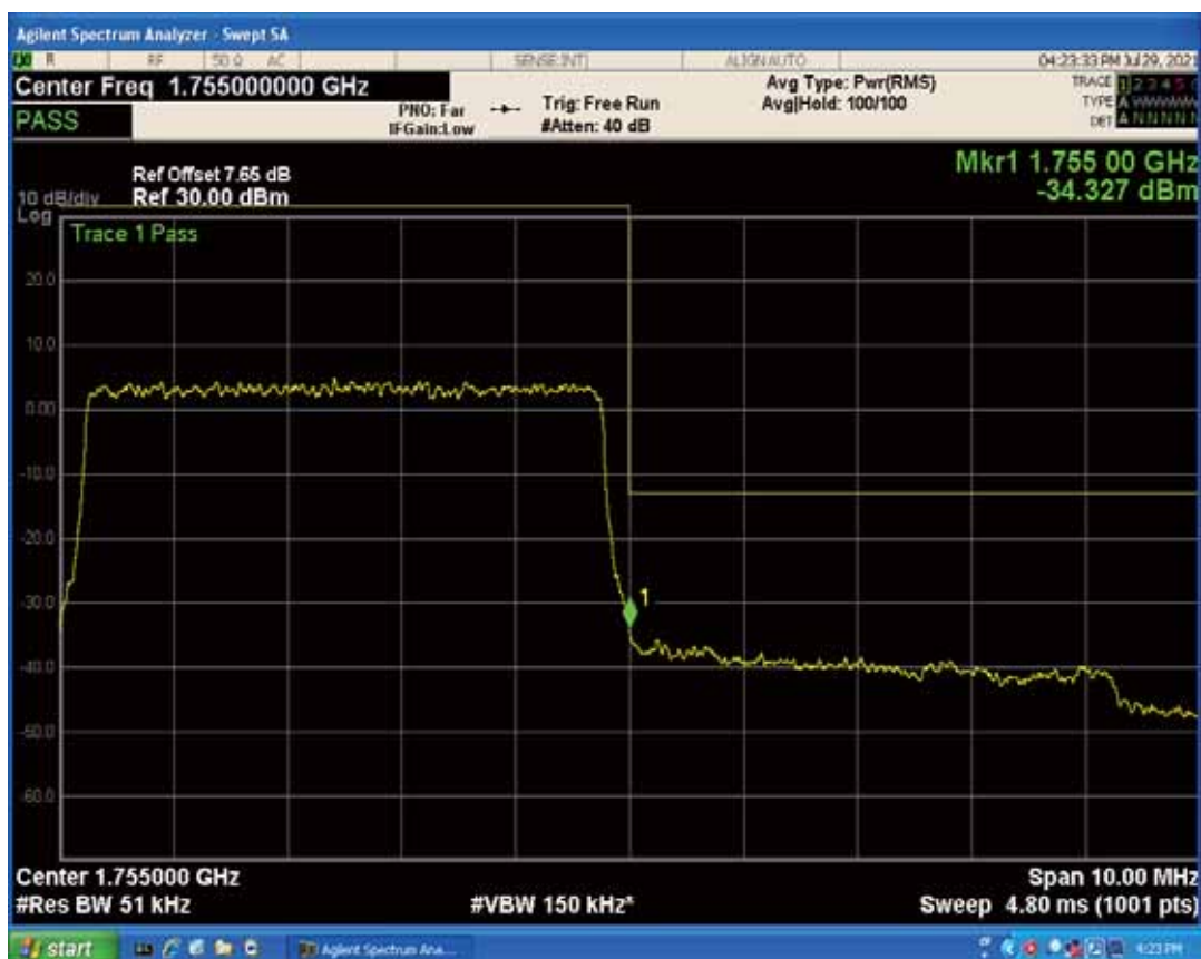
Band4 QAM16 BW=5MHz Channel=20375 RB Size=1 Position=#0
