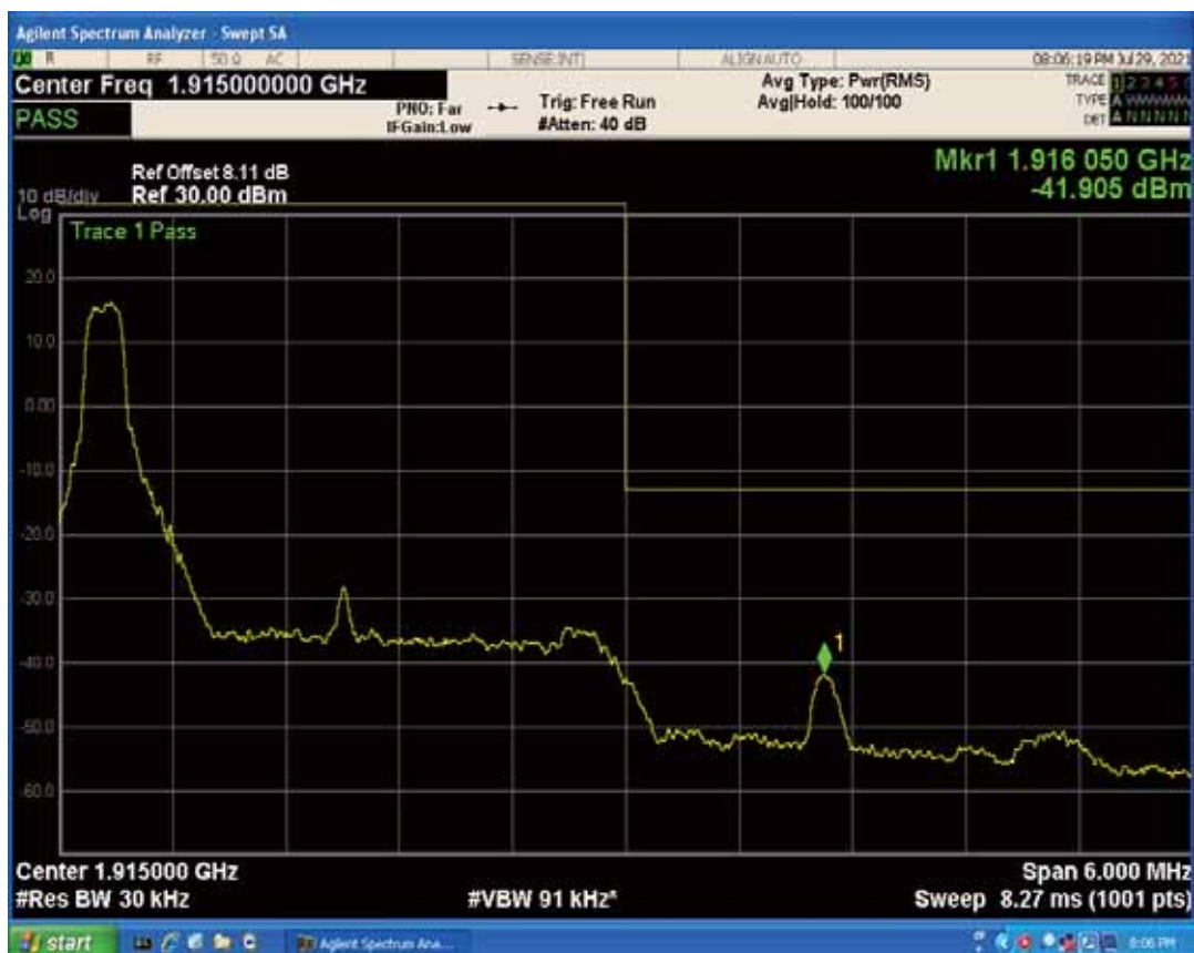
Band25 QAM16 BW=3MHz Channel=26055 RB Size=15 Position=#0
