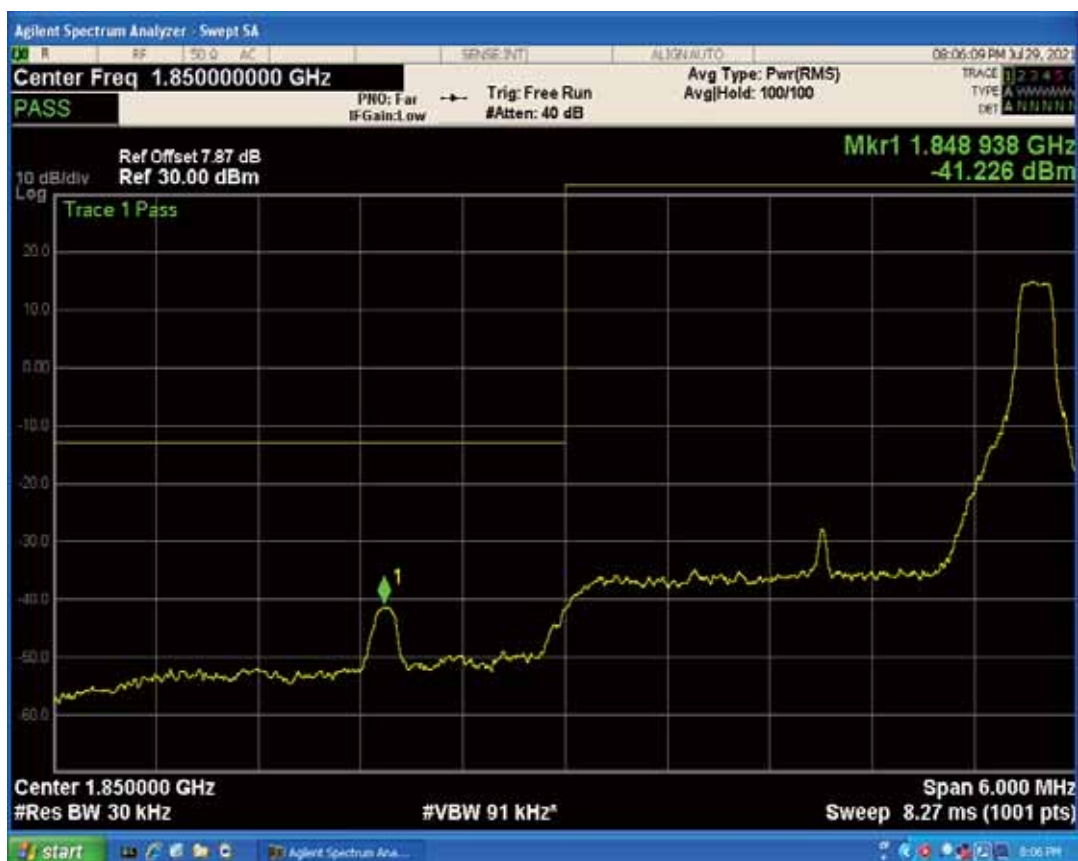
Band25 QPSK BW=3MHz Channel=26675 RB Size=1 Position=#0
