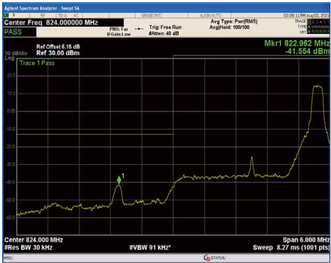
Band26b QAM16 BW=3MHz Channel=26805 RB Size=15 Position=#0
