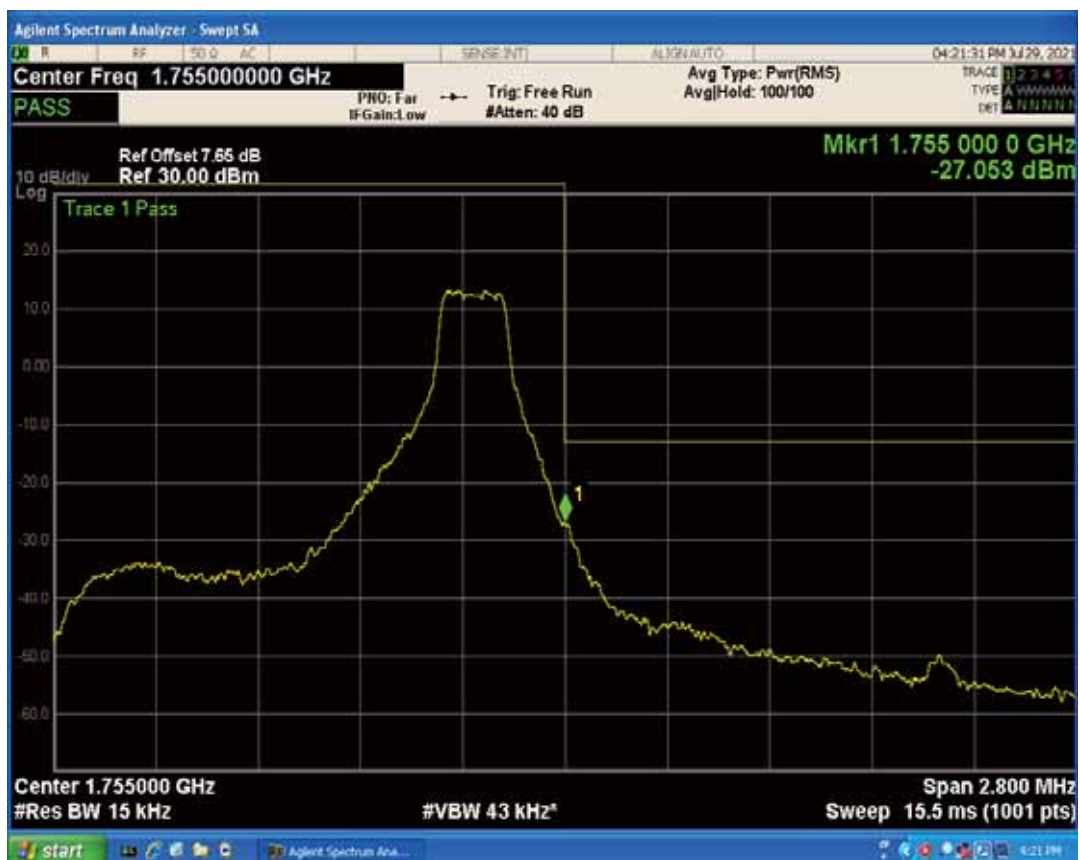
Band4 QPSK BW=1.4MHz Channel=20393 RB Size=6 Position=#0
