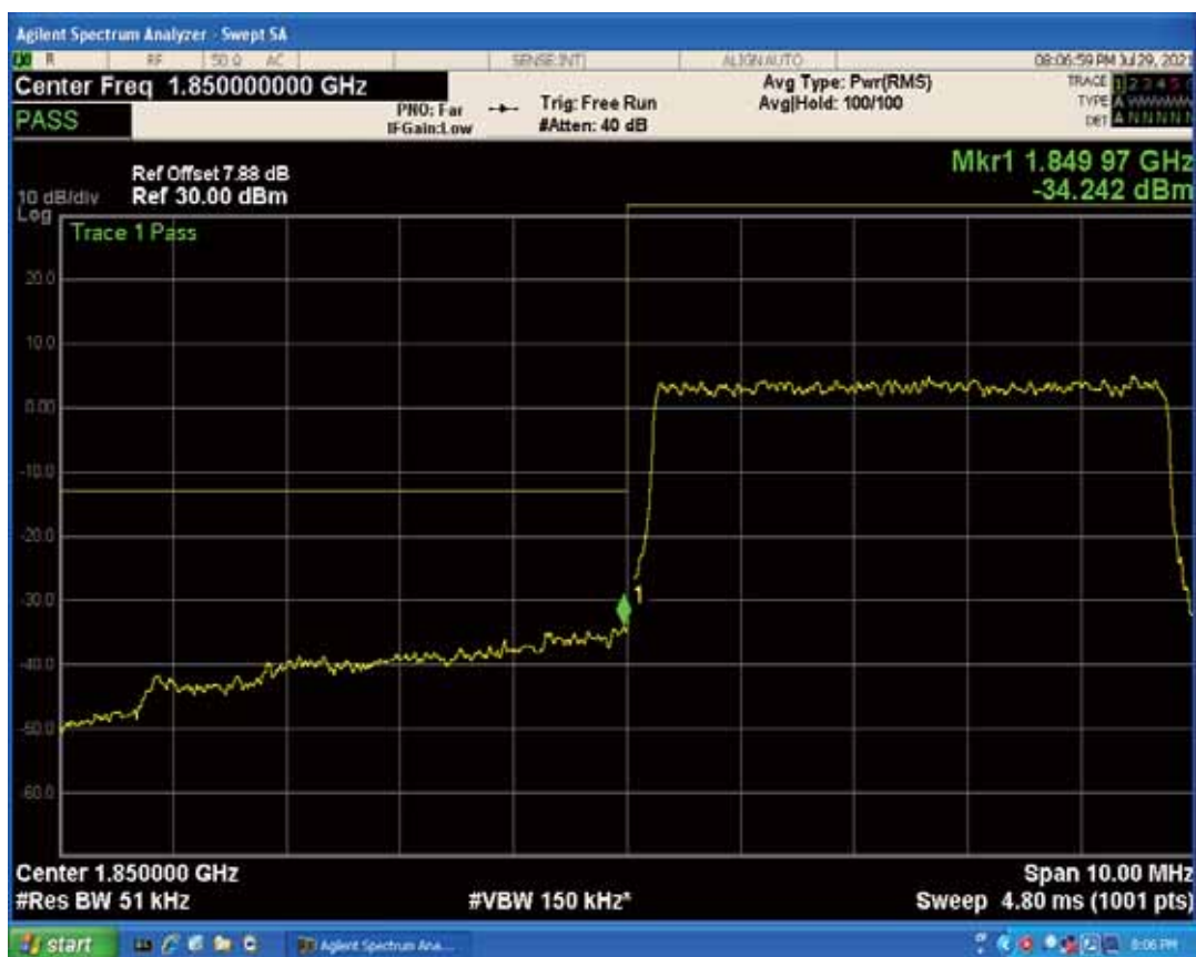
Band25 QAM16 BW=5MHz Channel=26065 RB Size=1 Position=#0
