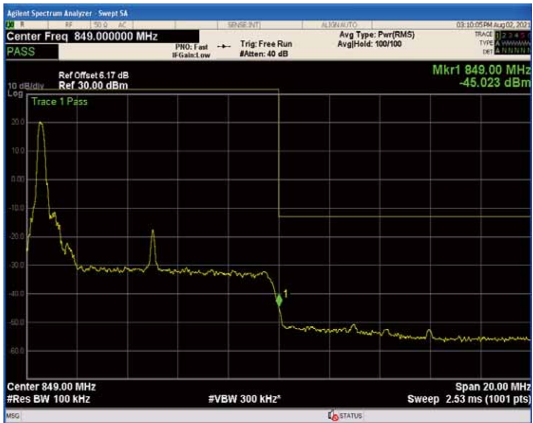
Band26b QPSK BW=10MHz Channel=26990 RB Size=50 Position=#0
