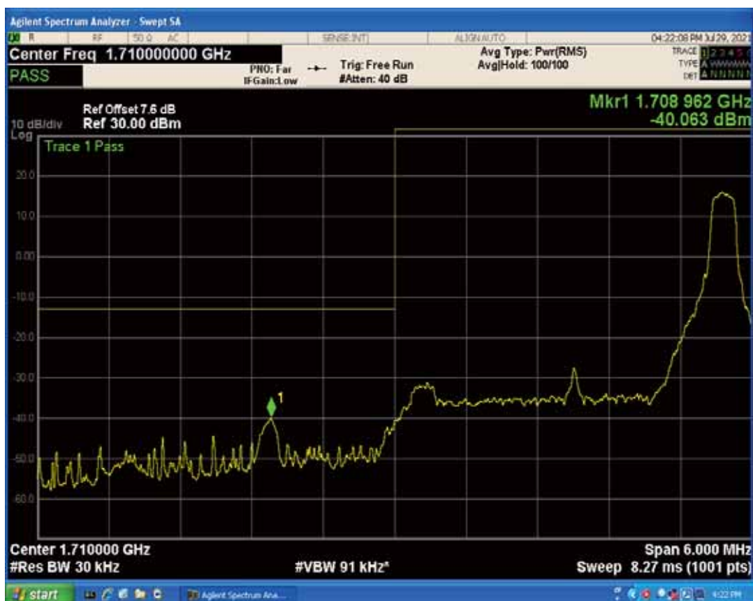
Band4 QPSK BW=3MHz Channel=19965 RB Size=1 Position=#0
