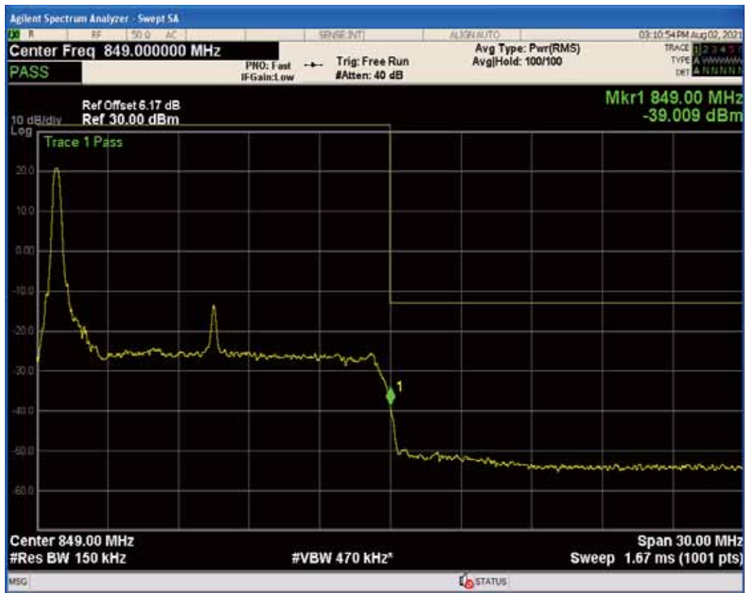
Band26b QPSK BW=15MHz Channel=26965 RB Size=1 Position=#Max
