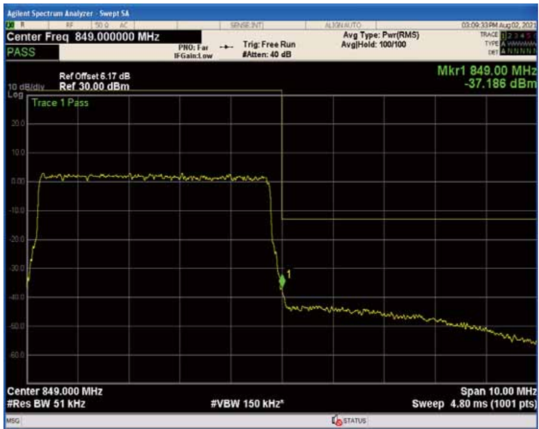
Band26b QAM16 BW=5MHz Channel=27015 RB Size=1 Position=#Max
