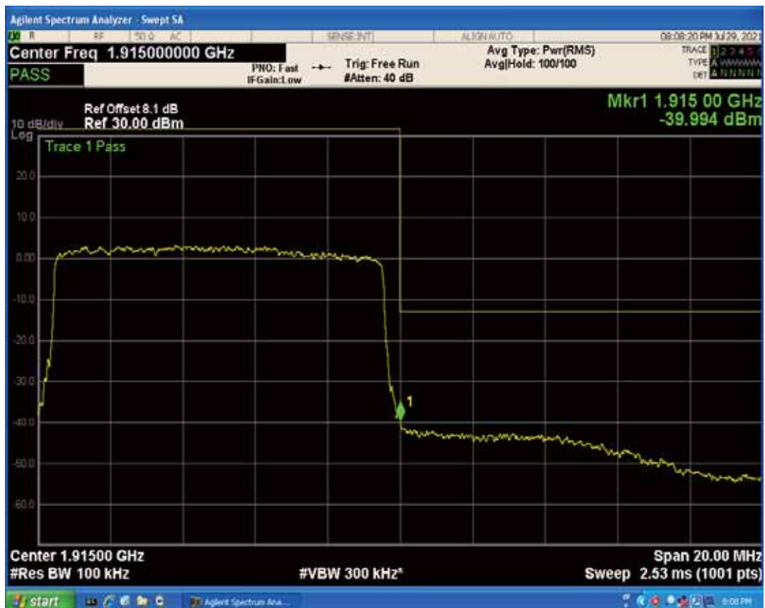
Band25 QPSK BW=15MHz Channel=26115 RB Size=1 Position=#0
