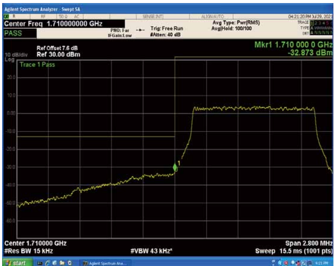
Band4 QPSK BW=1.4MHz Channel=20393 RB Size=1 Position=#0
