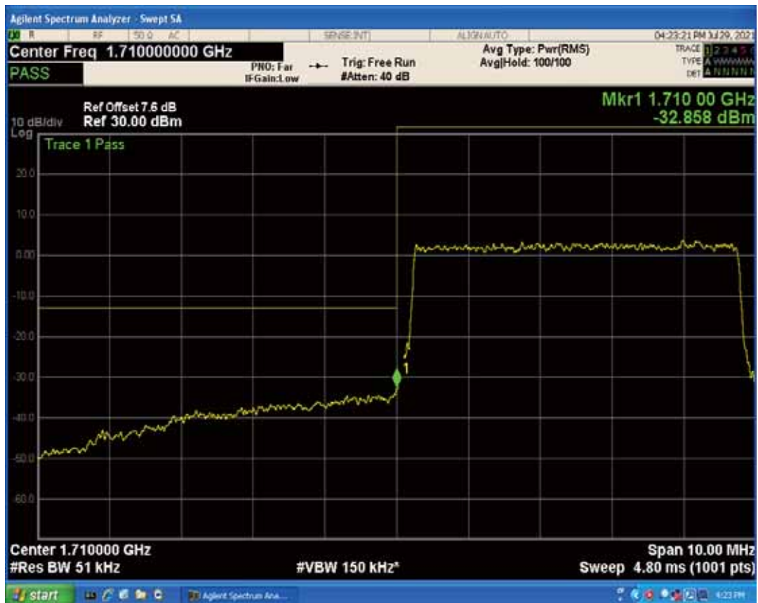
Band4 QPSK BW=5MHz Channel=20375 RB Size=1 Position=#Max
