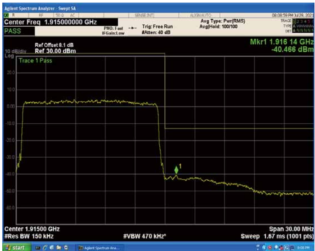
Band25 QAM16 BW=15MHz Channel=26615 RB Size=1 Position=#0
