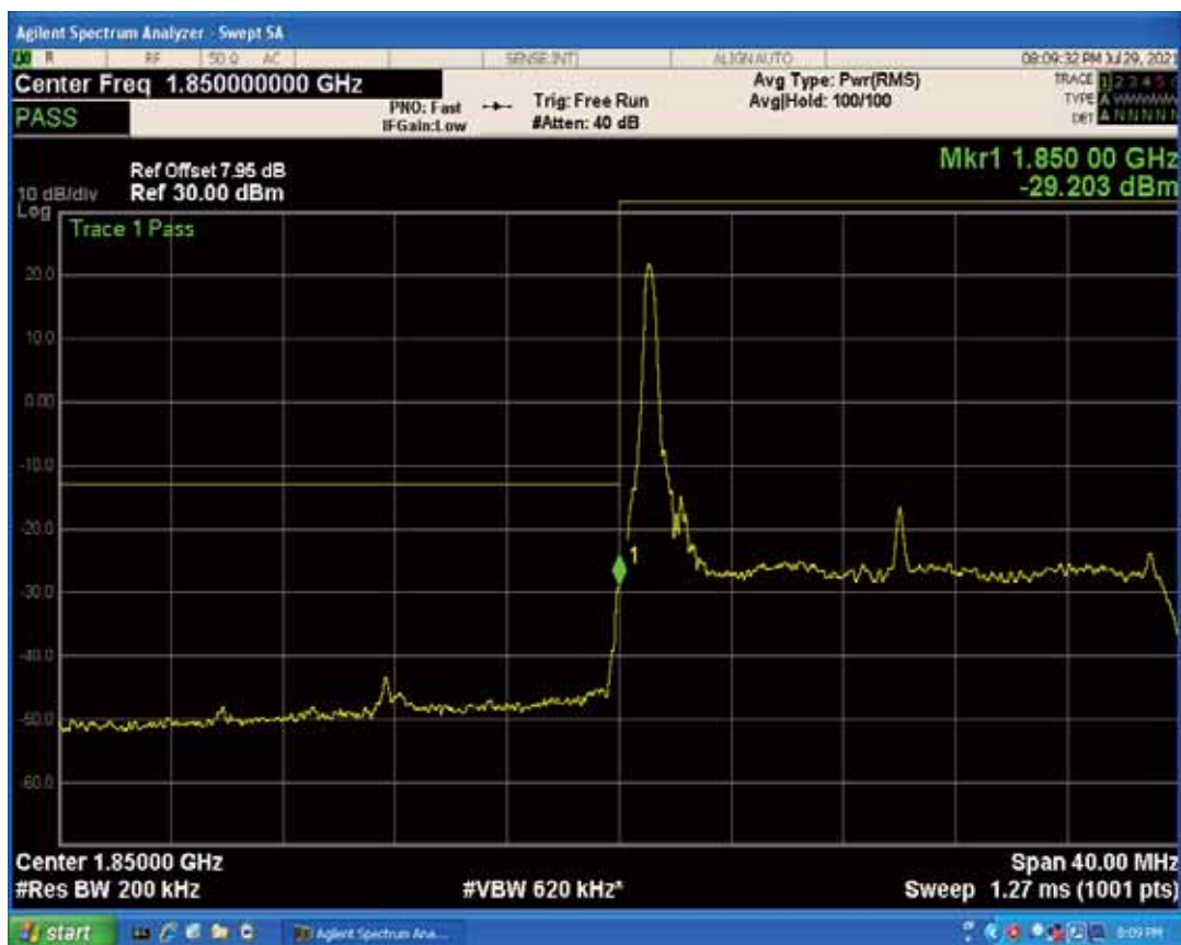
Band25 QAM16 BW=20MHz Channel=26140 RB Size=1 Position=#Max
