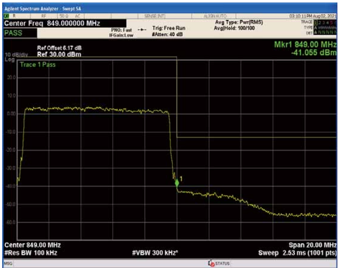
Band26b QPSK BW=10MHz Channel=26990 RB Size=1 Position=#Max
