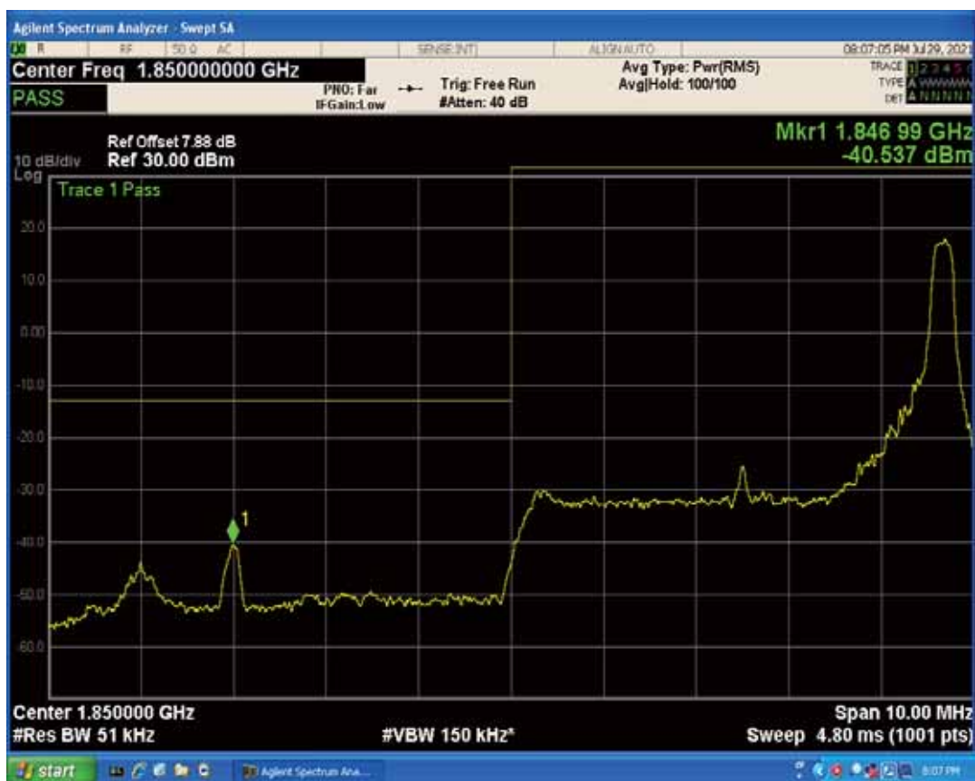
Band25 QAM16 BW=5MHz Channel=26065 RB Size=25 Position=#0
