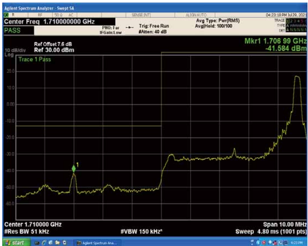
Band4 QPSK BW=5MHz Channel=20375 RB Size=1 Position=#0
