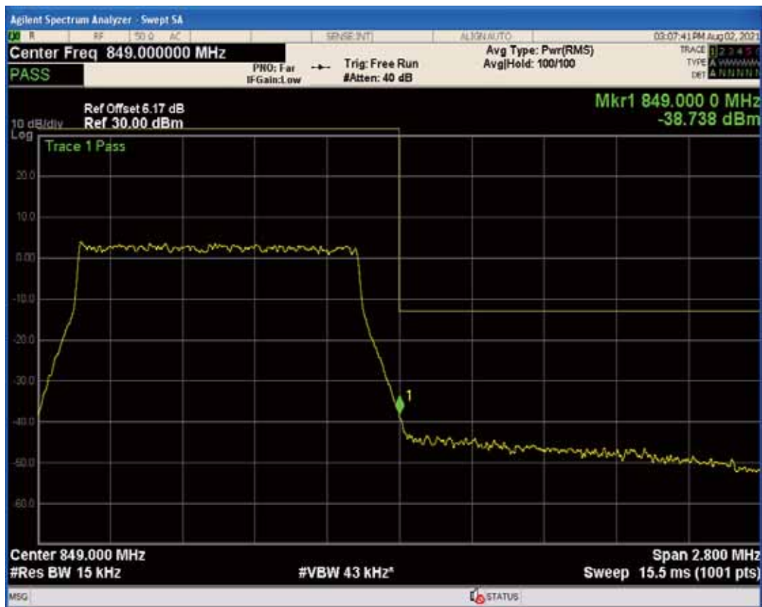
Band26b QPSK BW=3MHz Channel=26805 RB Size=1 Position=#0
