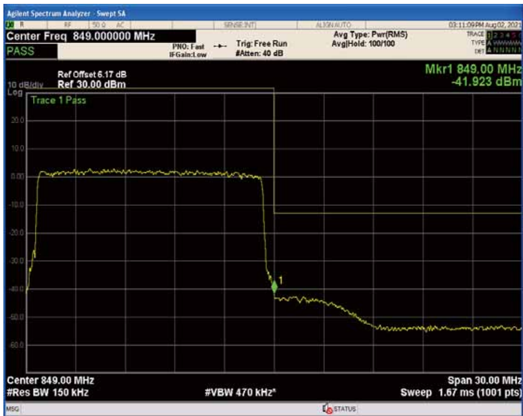
Band4 QPSK BW=1.4MHz Channel=19957 RB Size=1 Position=#Max
