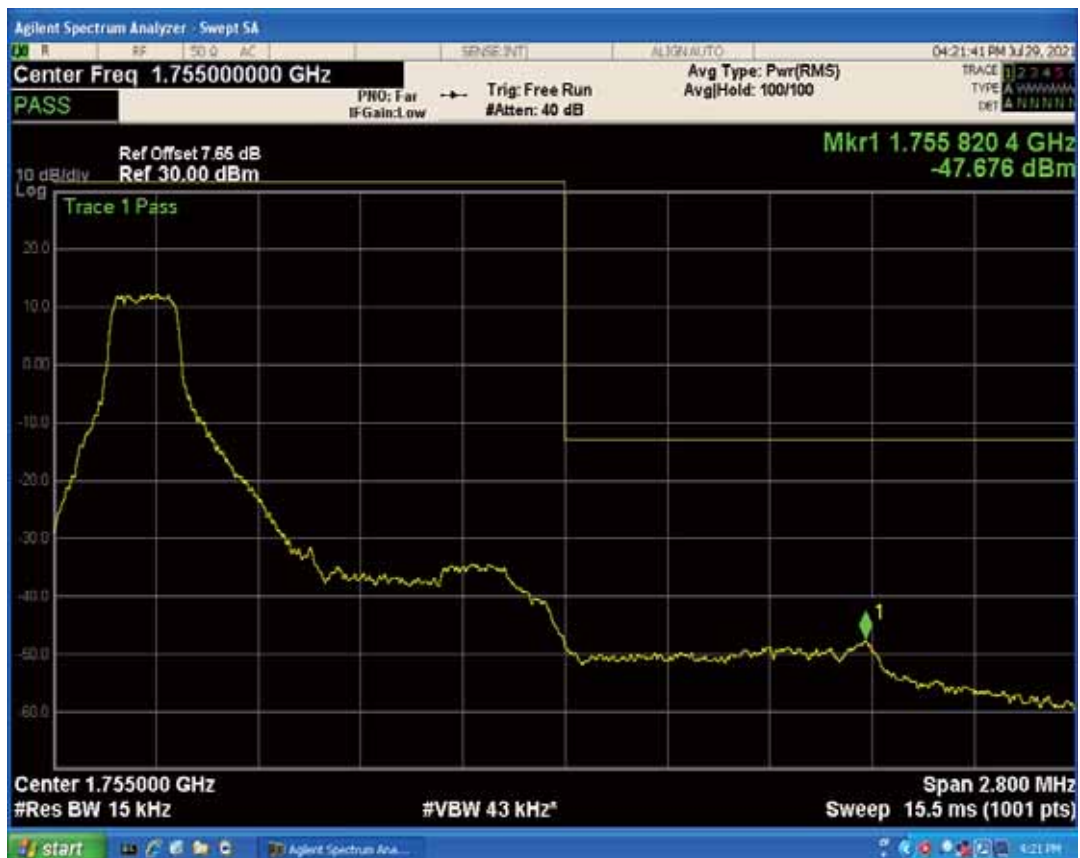
Band4 QAM16 BW=1.4MHz Channel=20393 RB Size=1 Position=#Max
