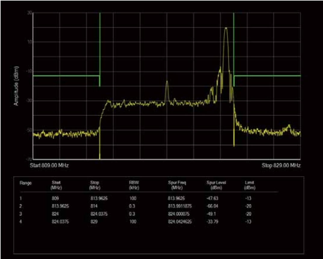
Band26a QPSK BW=10MHz Channel=26740 RB Size=1 Position=#0
