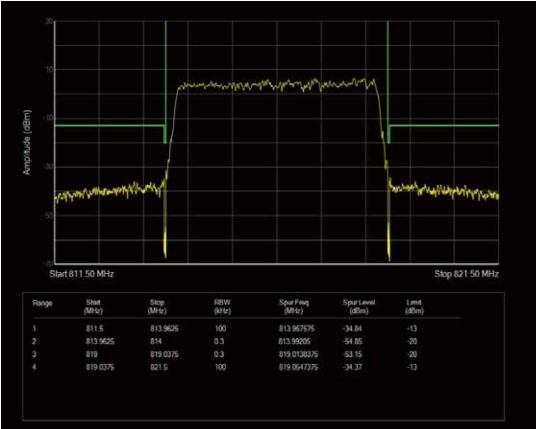
Band26a QAM16 BW=5MHz Channel=26715 RB Size=1 Position=#Max
