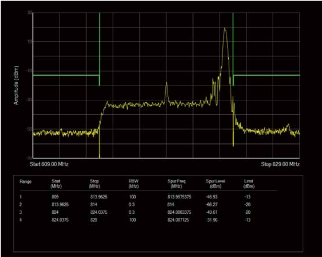
Band26a QAM16 BW=10MHz Channel=26740 RB Size=50 Position=#0
