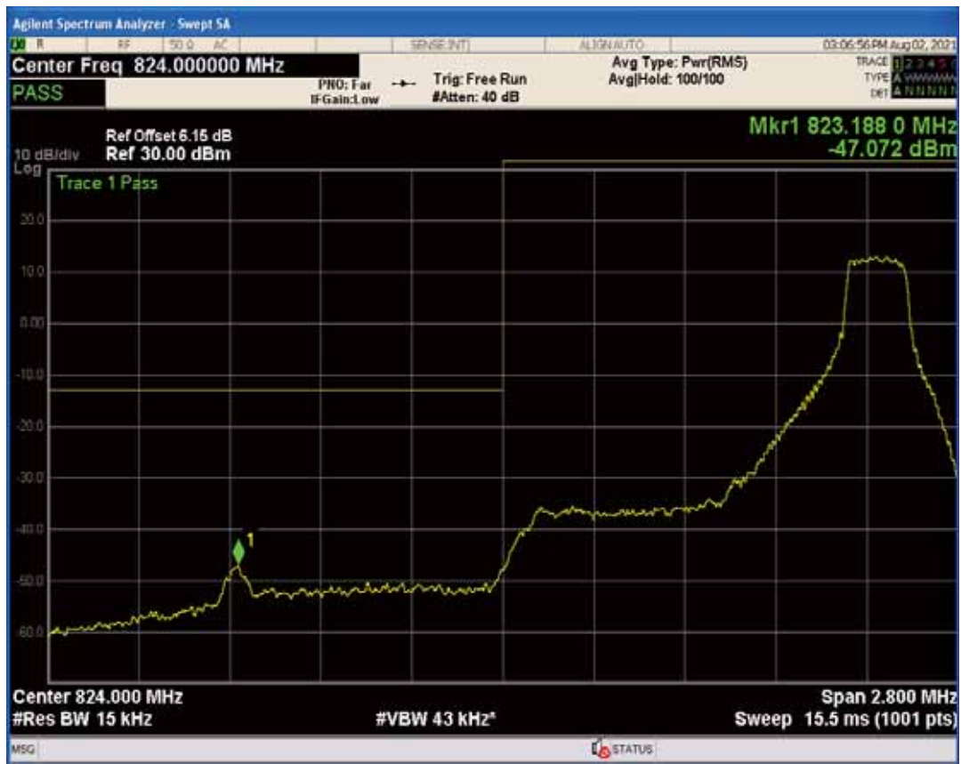
Band26b QAM16 BW=1.4MHz Channel=26797 RB Size=1 Position=#0
