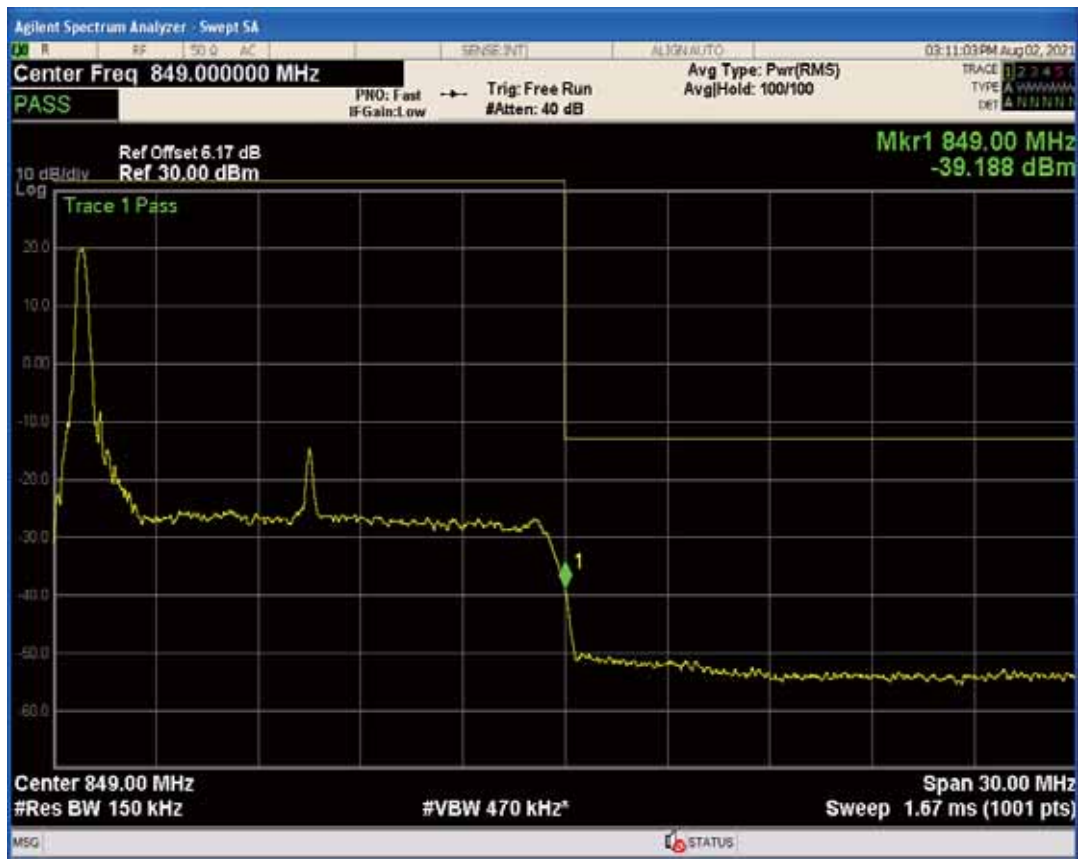
Band26b QAM16 BW=15MHz Channel=26965 RB Size=75 Position=#0
