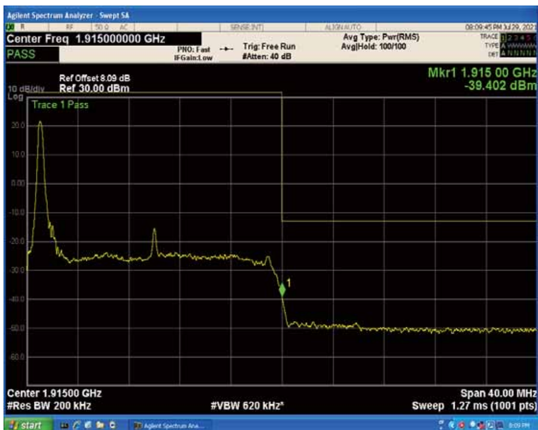
Band25 QPSK BW=20MHz Channel=26590 RB Size=1 Position=#Max
