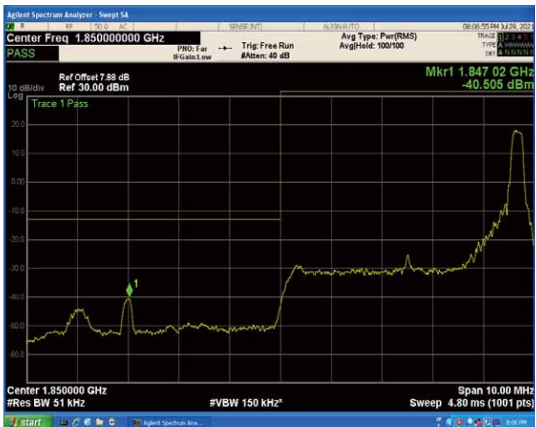
Band25 QPSK BW=5MHz Channel=26065 RB Size=25 Position=#0
