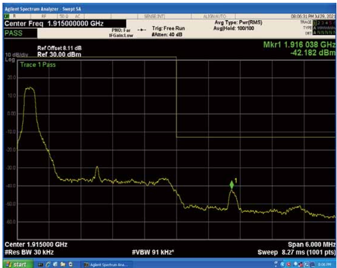
Band25 QPSK BW=3MHz Channel=26675 RB Size=15 Position=#0
