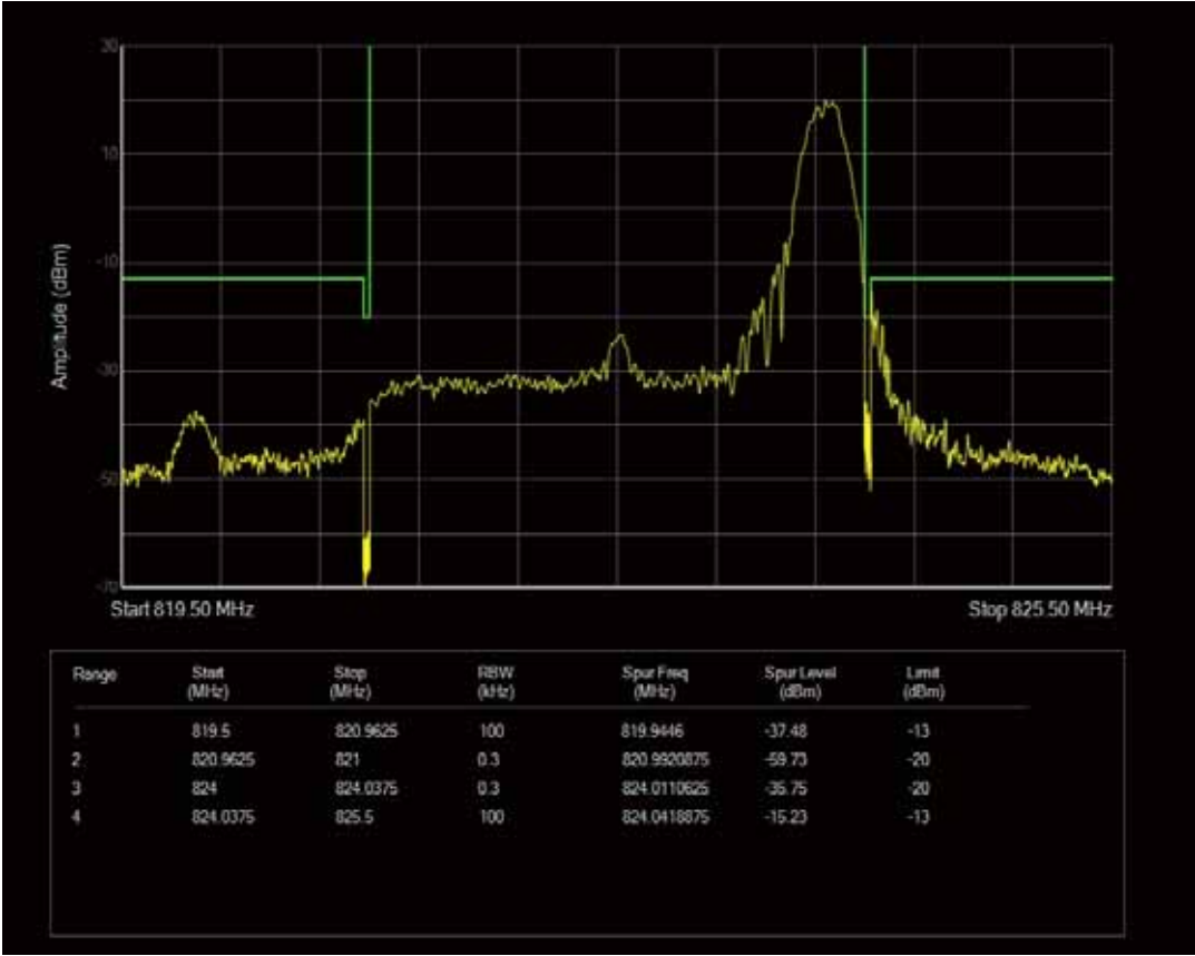
Band26a QPSK BW=5MHz Channel=26715 RB Size=1 Position=#0
