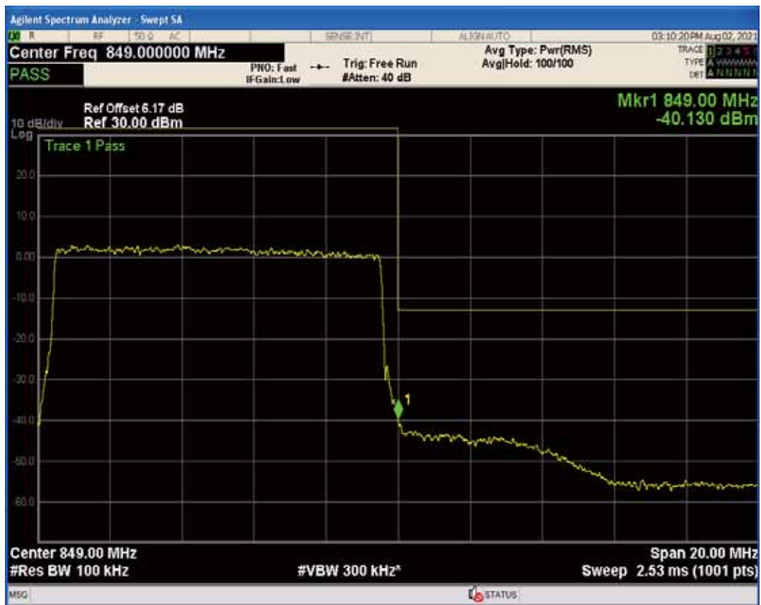
Band26b QPSK BW=15MHz Channel=26865 RB Size=1 Position=#Max
