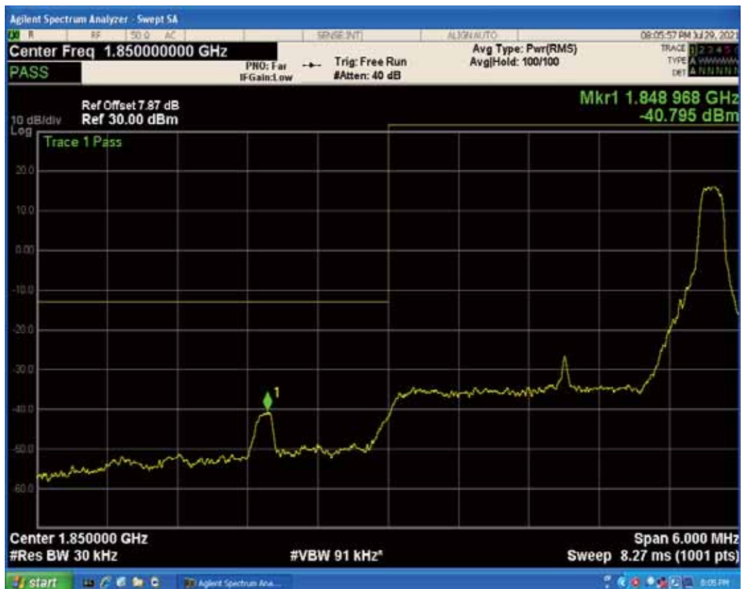
Band25 QAM16 BW=3MHz Channel=26055 RB Size=1 Position=#0
