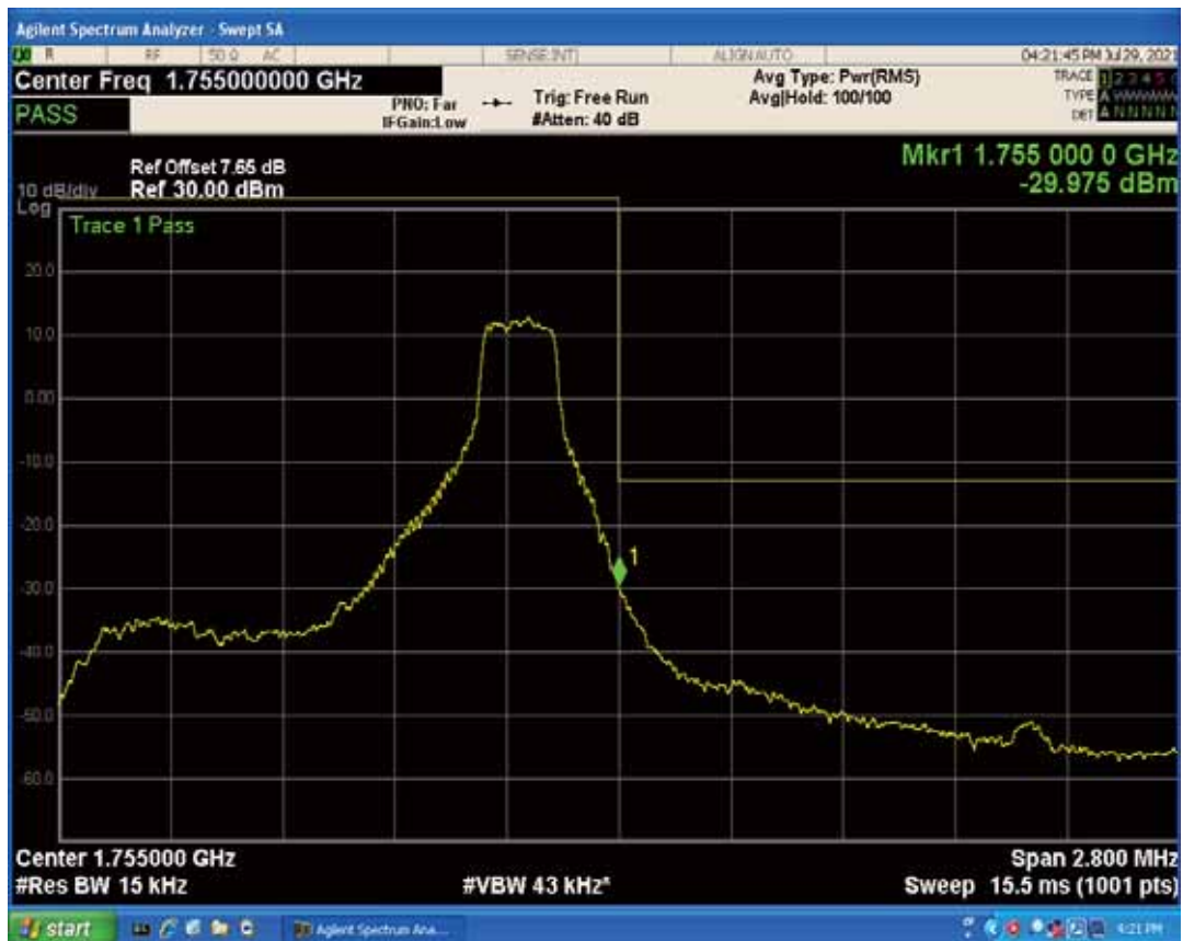
Band4 QAM16 BW=1.4MHz Channel=20393 RB Size=6 Position=#0
