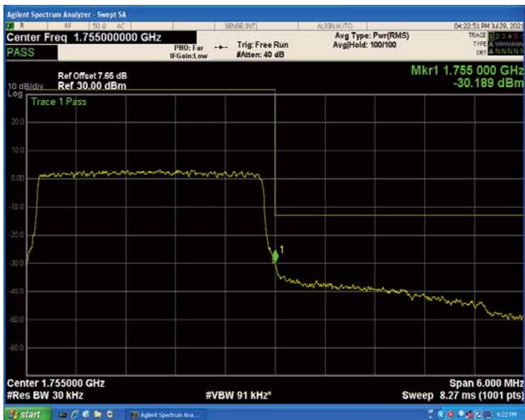
Band4 QPSK BW=5MHz Channel=19975 RB Size=1 Position=#0
