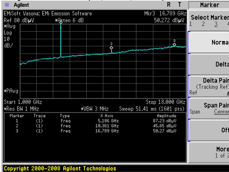
**Average Radiated Transmitter Spurs, 5220 MHz, 6 to 54 Mbps**
