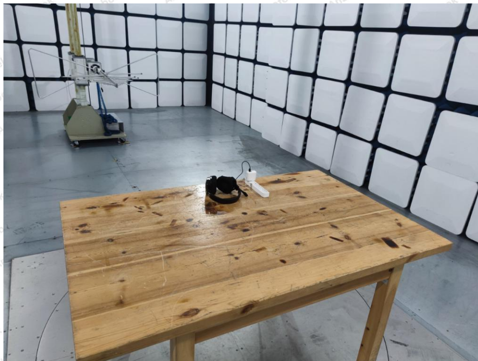
Photo of Radiation Emission Test
