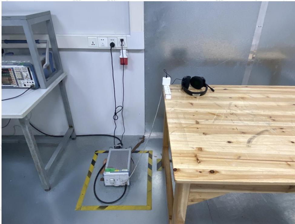
Photo of Conducted Emission Measurement
