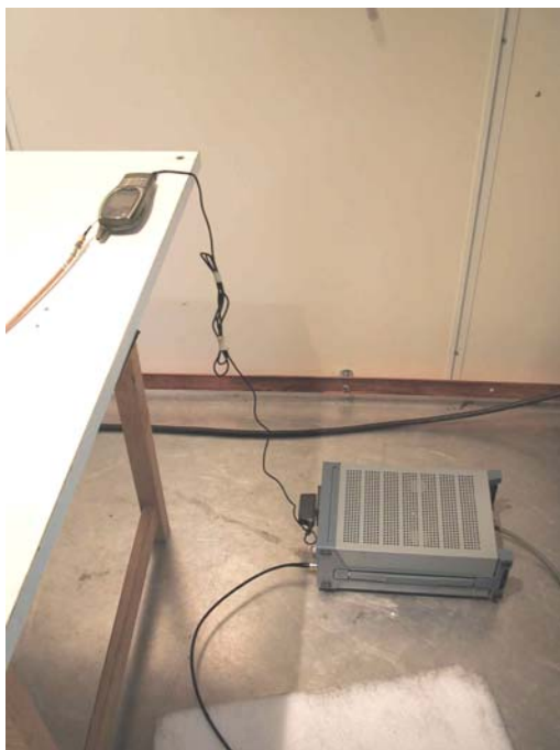
Picture 1: AC-power line conducted emissions test setup
