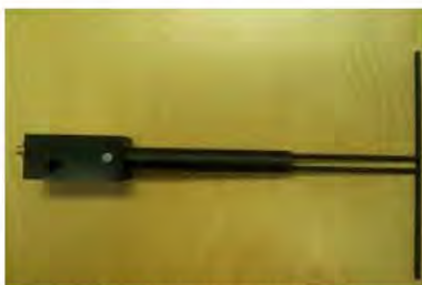
Figure 1 – MVG COMOSAR Validation Dipole
