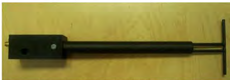
Figure 1 – MVG COMOSAR Validation Dipole
