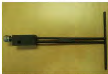
Figure 1 – MVG COMOSAR Validation Dipole
