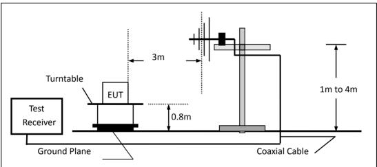
(c) For radiated emissions above 1000MHz
