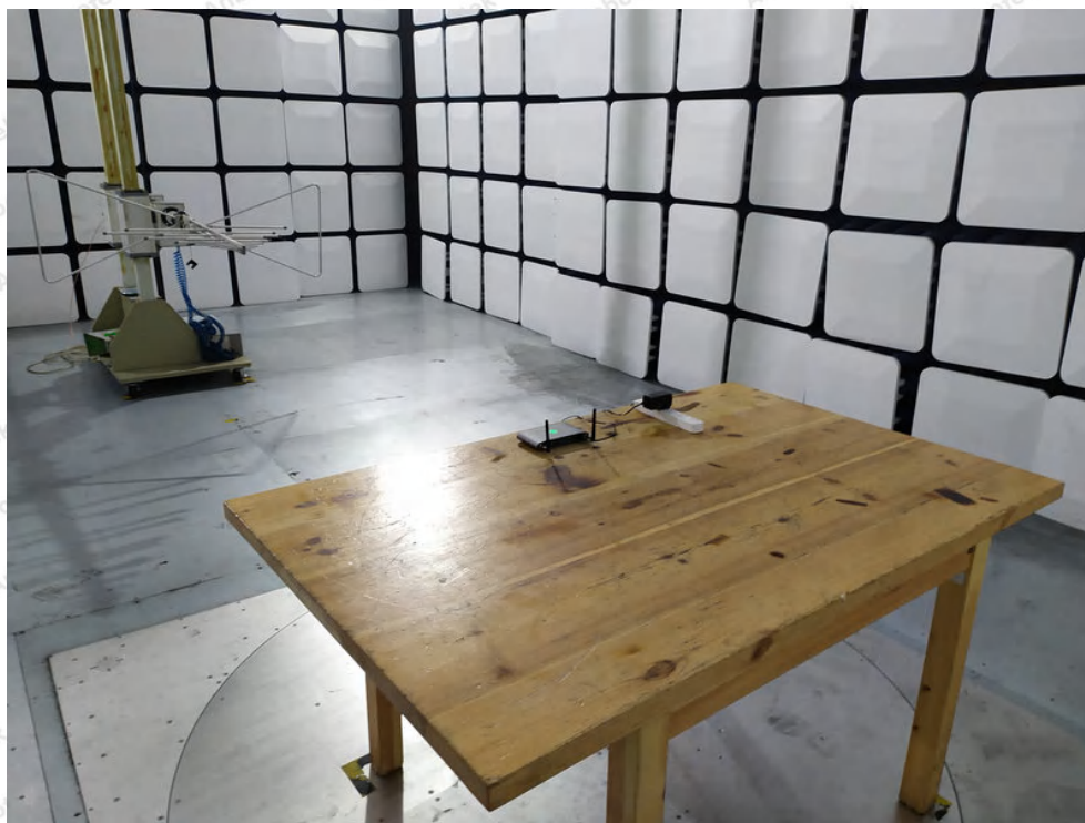
Photo of Radiation Emission Test
