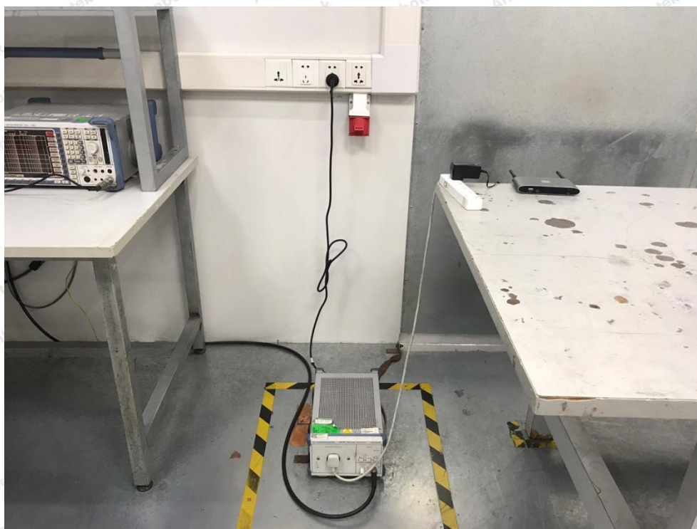
Photo of Power Line Conducted Emission Test
