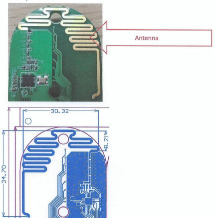
Antenna transmission frequency: 433.92MHz Antenna type: PCB Antenna
