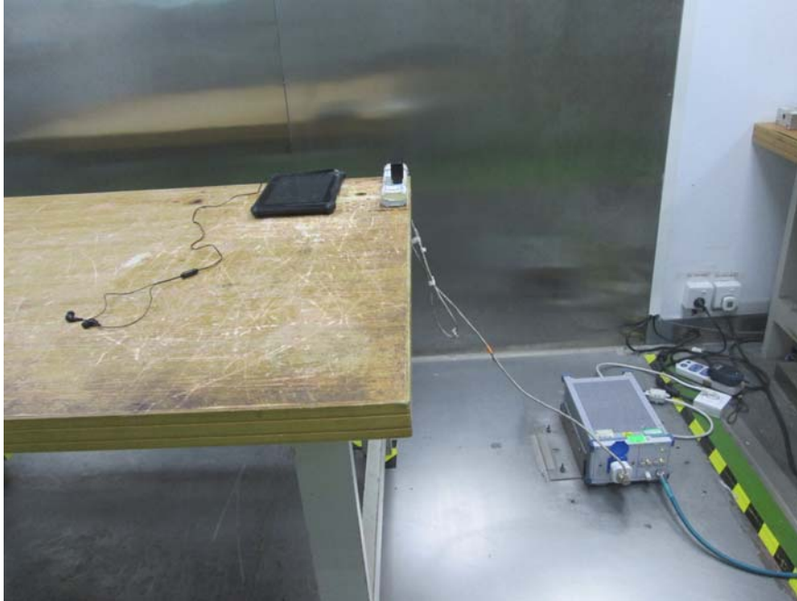
Conducted Emissions - Front View
