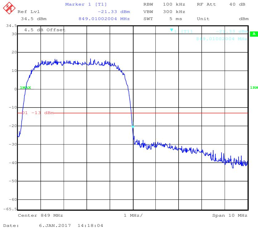
**PCS Band, Left Band Edge for GPRS Mode**
