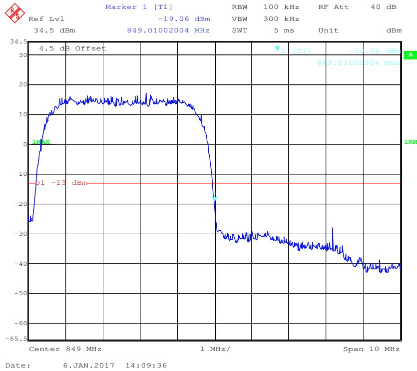
**Cellular Band, Left Band Edge for HSDPA (16QAM) Mode**
