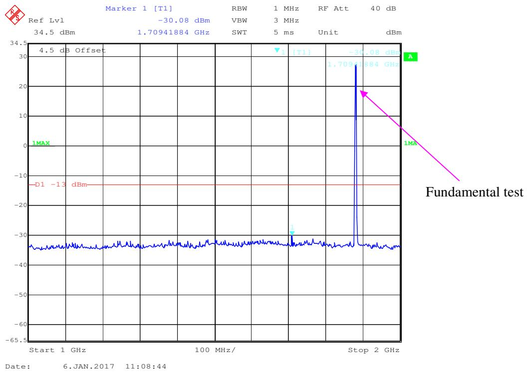
**2 GHz – 20 GHz (GPRS Mode)**
