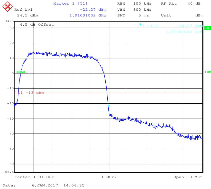
**PCS Band, Left Band Edge for HSDPA (16QAM) Mode**
