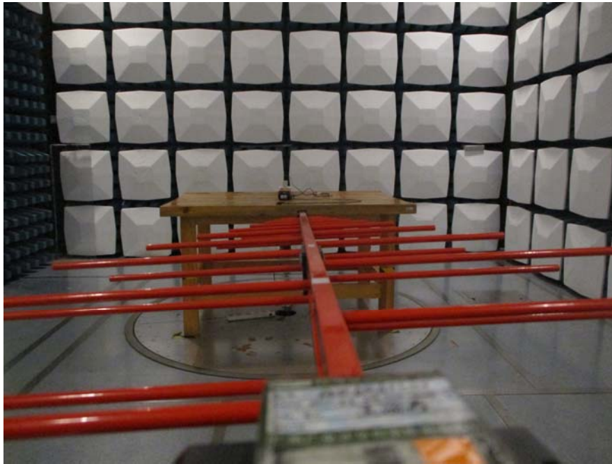
Radiated Emission View (Below 1GHz)
