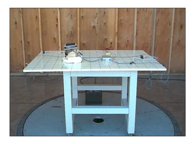
View of the Ignition Control System during the Radiated Emissions tests on the 10-Meter FCC listed OATS.
