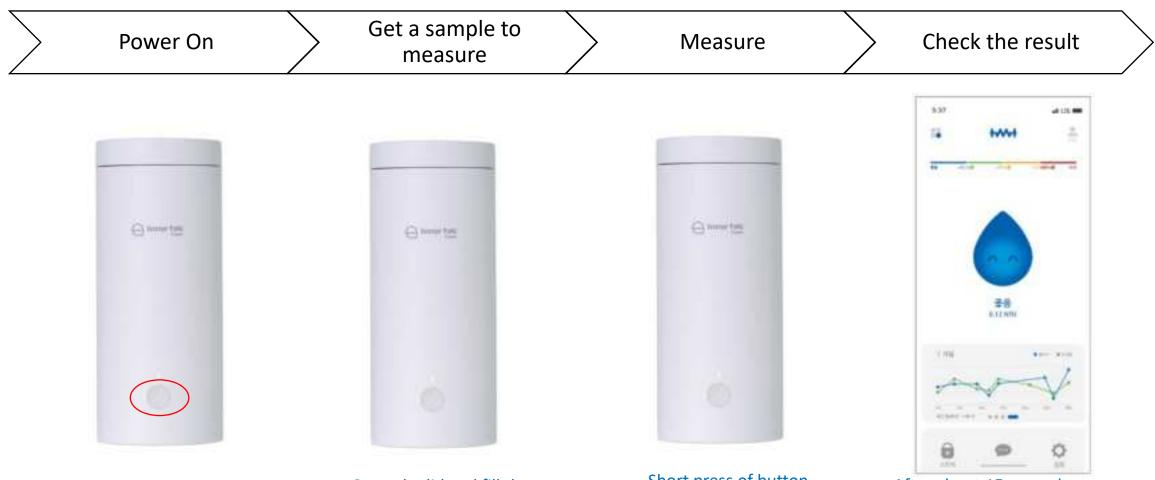
Power ON by pressing the button for more than 1.5 seconds Open the lid and fill the cup with water to be measured. Short press of button (less than 1.5 seconds) to start measurement
