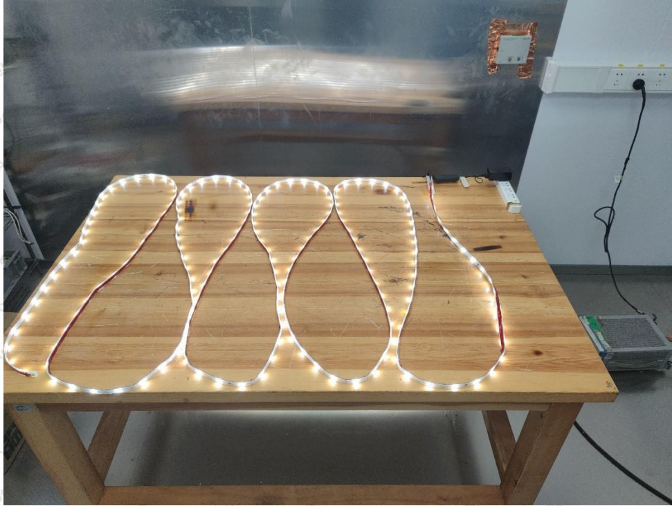
Photo of Radiation Emission Test (Below 1GHz)
