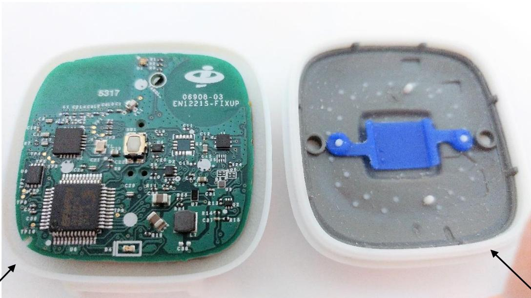
Bottom Housing      Primary Coin Cell Battery      **Bottom View**      Secondary Rechargeable Battery      Top Housing
