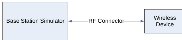
Figure 9-4 Power Measurement Setup
