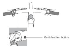
Gear shift: Short press the Multi-function button twice to shift 0-3 gear;
