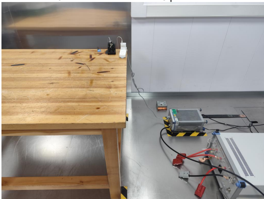
Conducted Emission at AC power line
