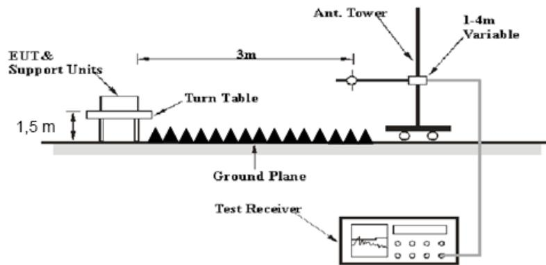
The radiated emissions were performed in the 3 meters distance, using the setup accordance with the ANSI C63.10-2013. The specification used was the FCC 15.209, and FCC 15.247 limits.
