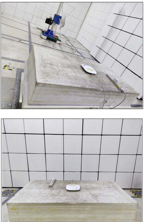
Radiated Emission Test (Below 1GHz) (Test Mode A)
