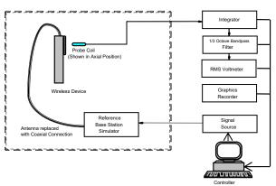
Figure 4-13 **Audio Magnetic Field Test Setup**
