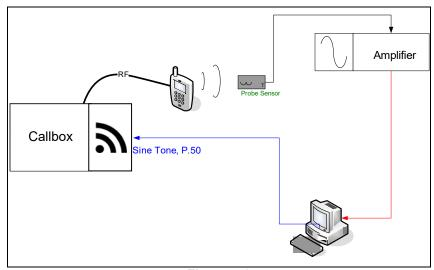
Figure 4-2 T-Coil Test Setup
