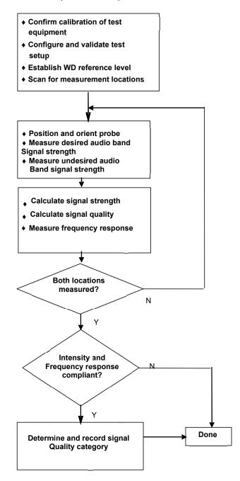
Figure 4-14 C63.19 T-Coil Signal Test Process
