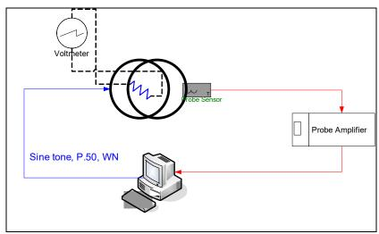
Figure 4-1 Validation Setup with Helmholtz Coil
