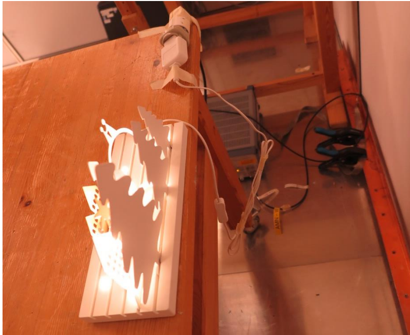
Test setup for conducted emission 150 kHz – 30 MHz
