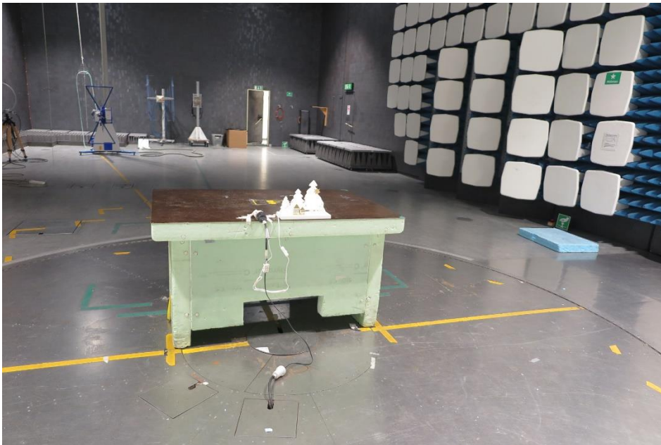
Test set up radiated emission 30 MHz – 1 GHz
