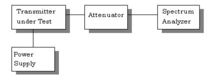
**METHOD OF MEASUREMENT:** The procedure used was EIA/TIA-382-A.
