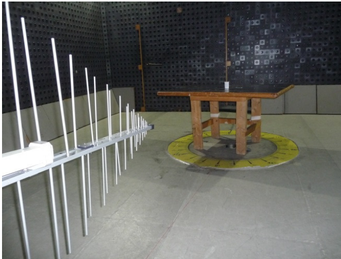
Photograph 8.1.1 Setup for radiated emission measurements
