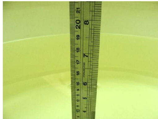
Fig 7.2 Photo of Liquid Height for Body SAR
