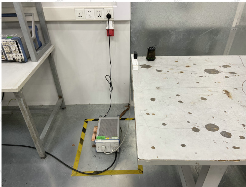
Photo of Power Line Conducted Emission Test
