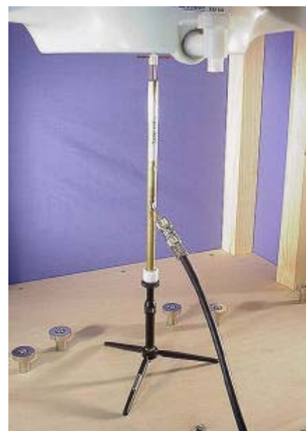
2450MHz System Check Setup Photograph
