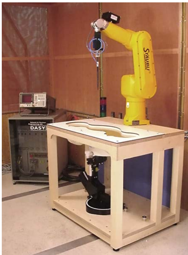
DASY3 SAR Measurement System with SAM phantom
