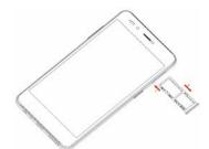
make sure that the clipped corner of your SIM card is facing the correct direction, Keep the SIM cards into the given SIM slots, then Push the SIM Tray inside as shown below. Follow the same method for inserting your SD Card.
