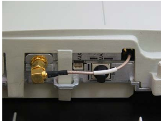
Fig.1 – RF power selector rotary switch
