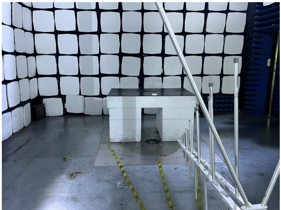
Radiation Emission Test Setup (30MHz to 1GHz)
