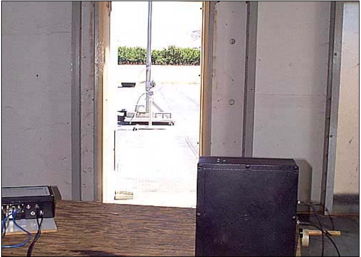
Radiated Emissions - Back View Close-up with Mag Loop Antenna
