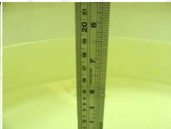
Photo of Liquid Height for Body SAR
