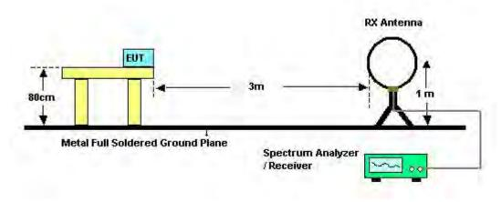
For Radiated Emissions: 30MHz~1GHz
