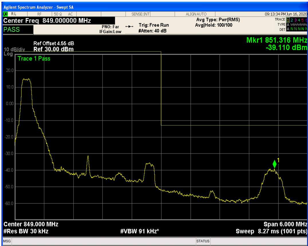
LTE Band5 QAM16 BW=3MHz Channel=20635 RB Size=1 Position=#Max
