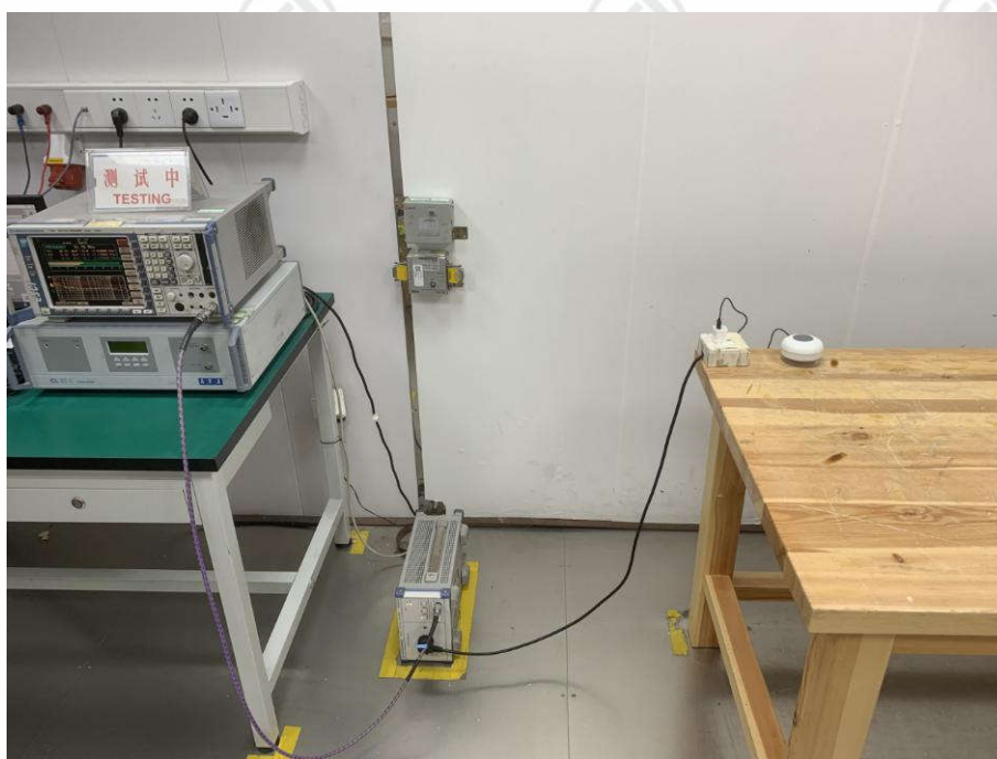
CONDUCTED EMISSION TEST SETUP
