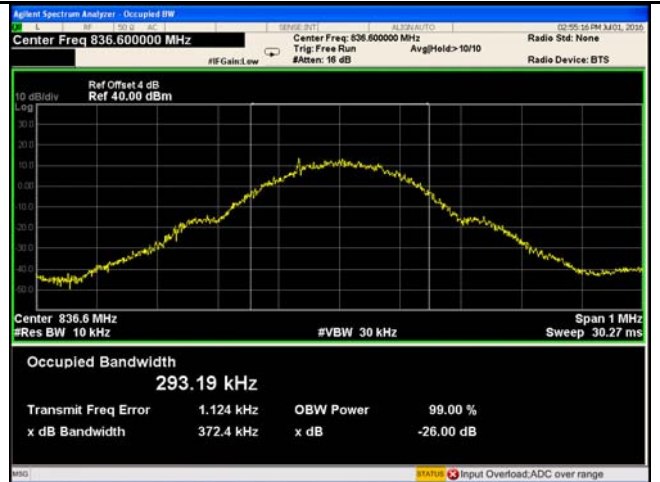
GSM 850 BW - Mid CH 836.6MHz
