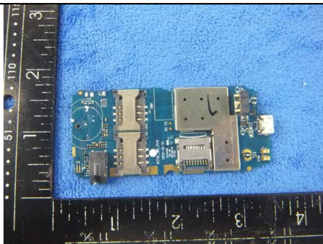
Mainboard with Shielding - Front View
