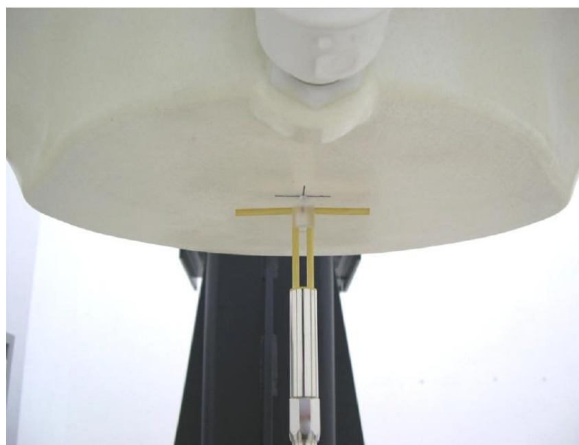
Picture 8.2 Photo of Dipole Setup
