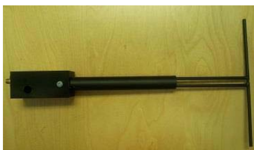
Figure 1 – MVG COMOSAR Validation Dipole
