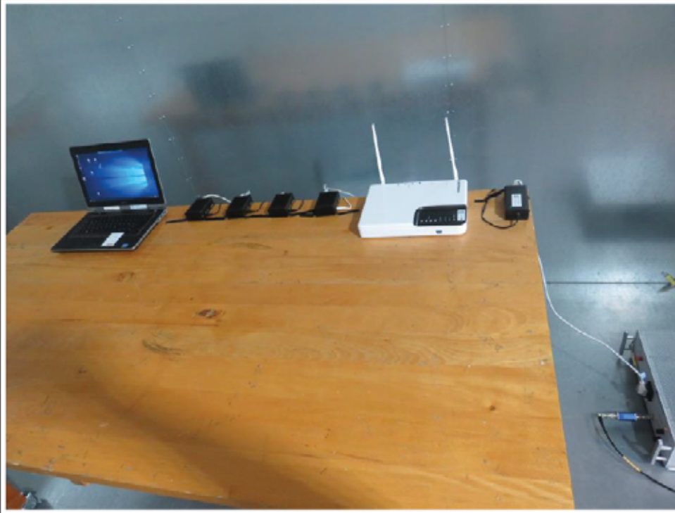
TEST SETUP EUT WITH AE ON TABLE
