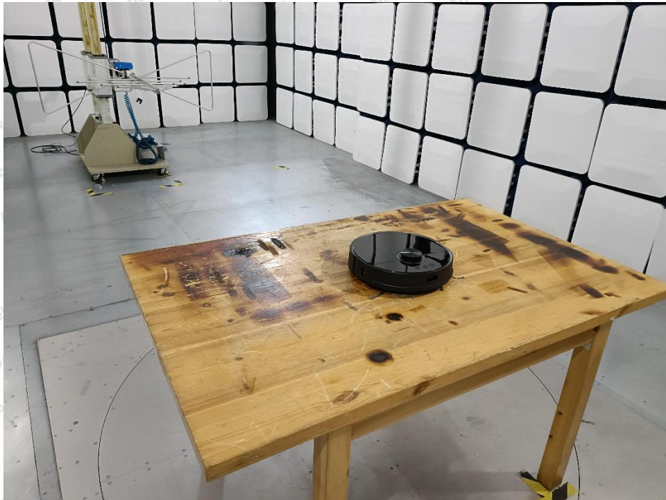
Photo of Radiation Emission Test
