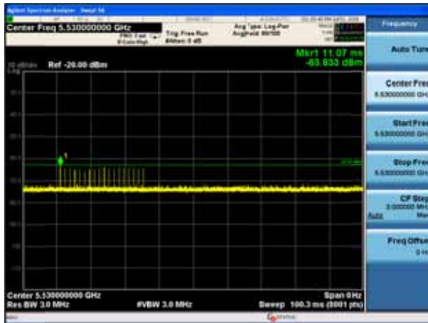
11ac80 CH106 5530MHz Radar Type 2 Calibration Plot
