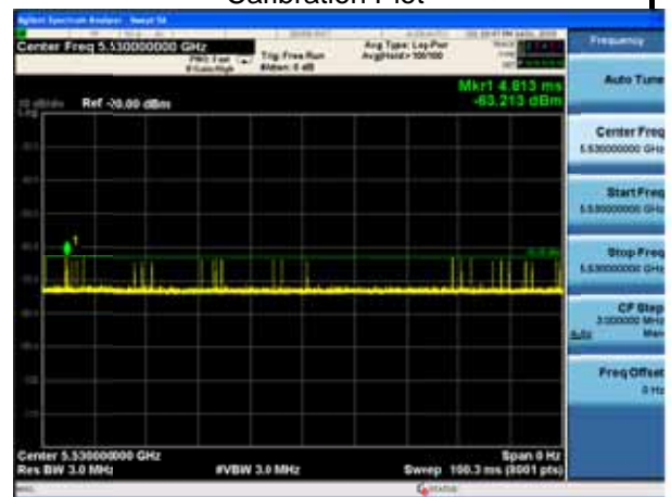
11ac80 CH106 5530MHz Radar Type 5 Calibration Plot
