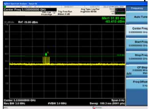
11ac80 CH106 5530MHz Radar Type 3 Calibration Plot
