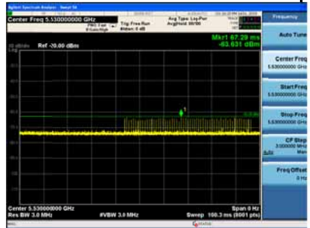
11ac80 CH106 5530MHz Radar Type 3 Calibration Plot
