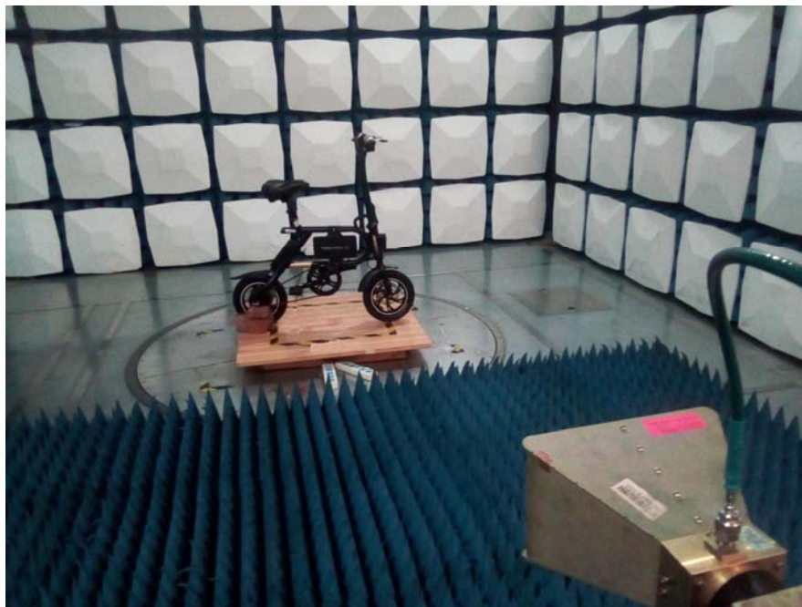
Radiated Emission Above 1GHz View
