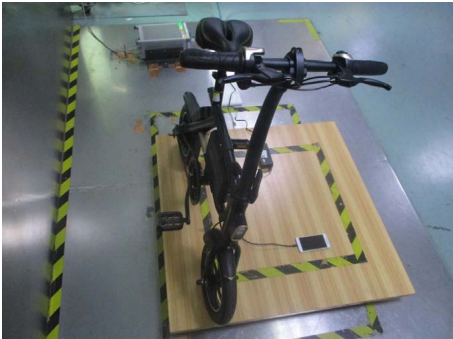
Conducted Emissions Side View
