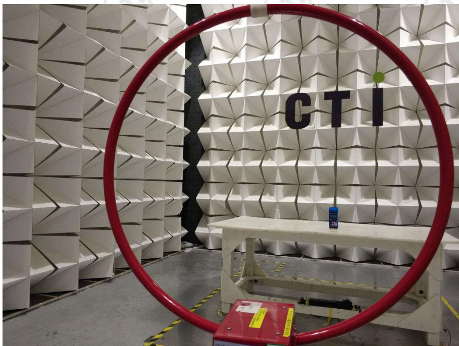
Radiated spurious emission Test Setup-1(Below 30MHz)
