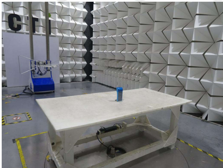
Radiated spurious emission Test Setup-2(Below 1G)
