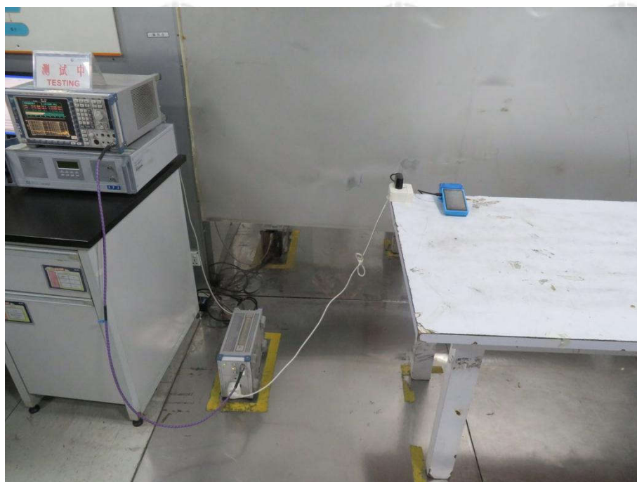
Conducted Emissions Test Setup
